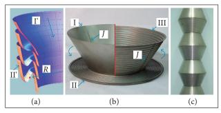
**Figure 1.** Graphic representation of the mathematical model for: (a) Fragment transformation of the initial conical shell (I') into a single corrugation (II'); (b) The transformation stages of the metal TVS shell; (c) Design solution for multi-conical TVS. J represents the welded joints of the shells.
