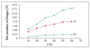
**Figure 5.** The number of fringes N in a shearographic interferogram depending on the time of radiation heating t in a TVS shell part.
