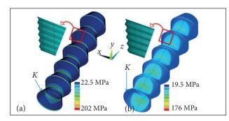
**Figure 3.** Equivalent stresses  $\sigma_e$  in TVS with a piecewise smooth (a) and sinusoidal (b) profiles of the shell meridian subjected to the effect of maximum SEF values.
