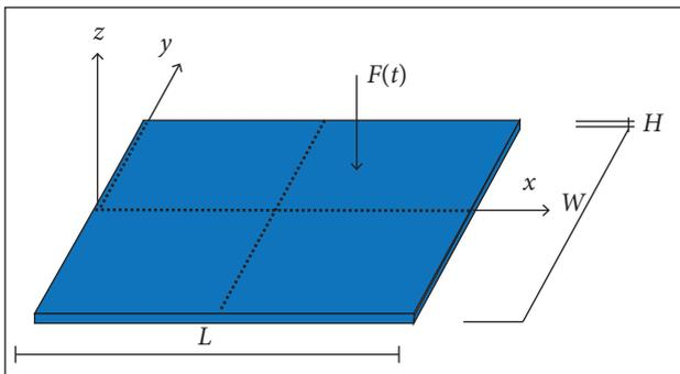
**Figure 1.** Geometry of the considered laminated composite plate.
