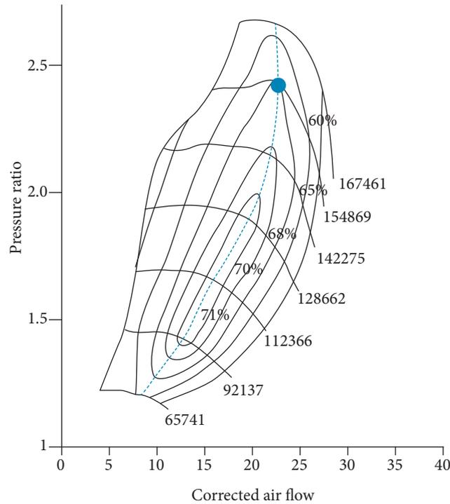
**Figure 13.** The optimized high pressure turbocharger compressor map.
