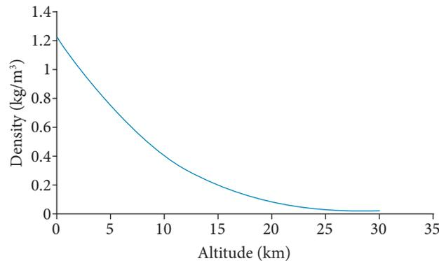
**Figure 1.** Diagram of air density variation with altitude.
