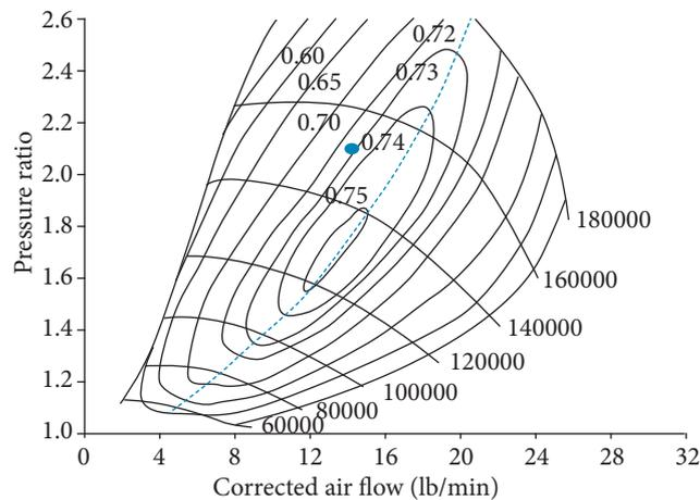
**Figure 8.** Compressor map of the well-chosen turbocharger.
