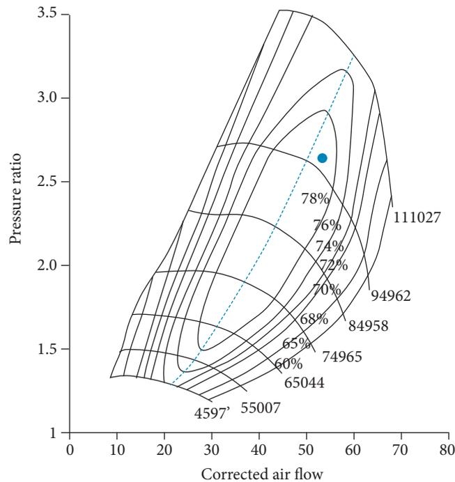
**Figure 12.** The optimized intermediate pressure turbocharger compressor map.
