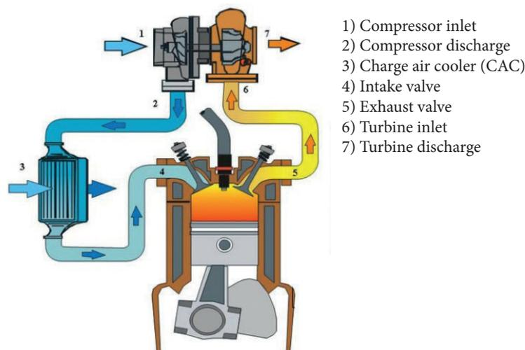
**Figure 2.** Schematic of a turbocharged engine.
