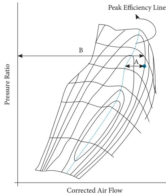
**Figure 5.** Dimensionless distance from peak efficiency line.
