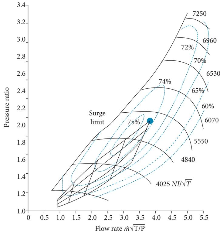
**Figure 4.** Matching of engine and compressor maps.
