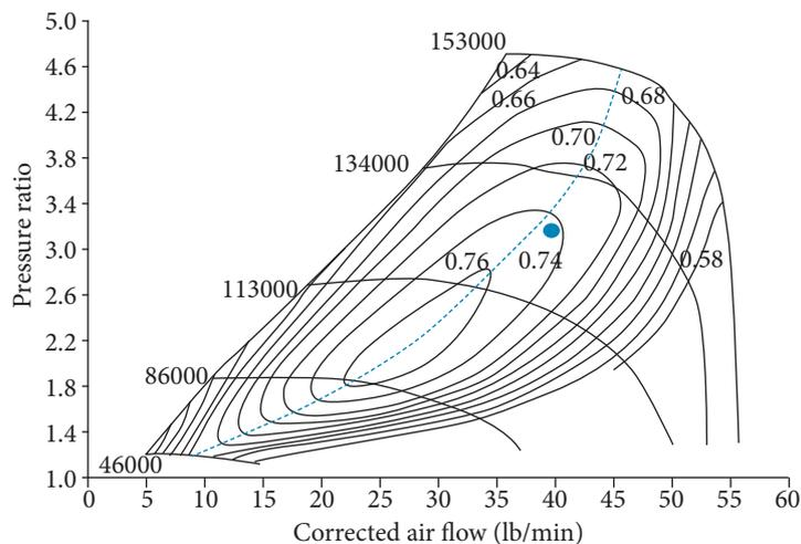
**Figure 9.** The optimized low pressure turbocharger compressor map.
