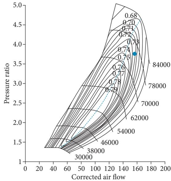
**Figure 11.** The optimized low pressure turbocharger compressor map.
