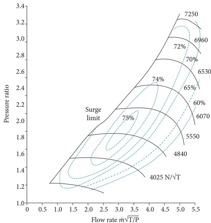
**Figure 3.** An example of the turbocharger compressor map.
