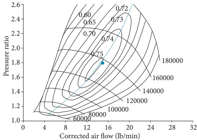
**Figure 10.** The optimized high pressure turbocharger compressor map.
