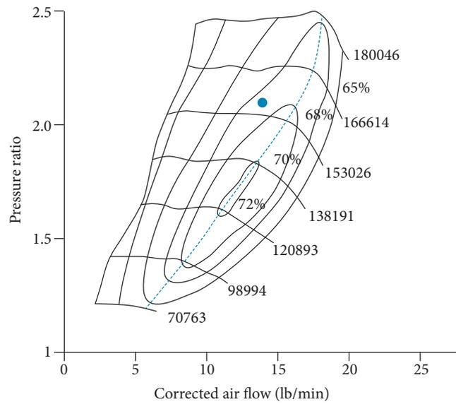
**Figure 7.** Compressor map of the well-chosen turbocharger.
