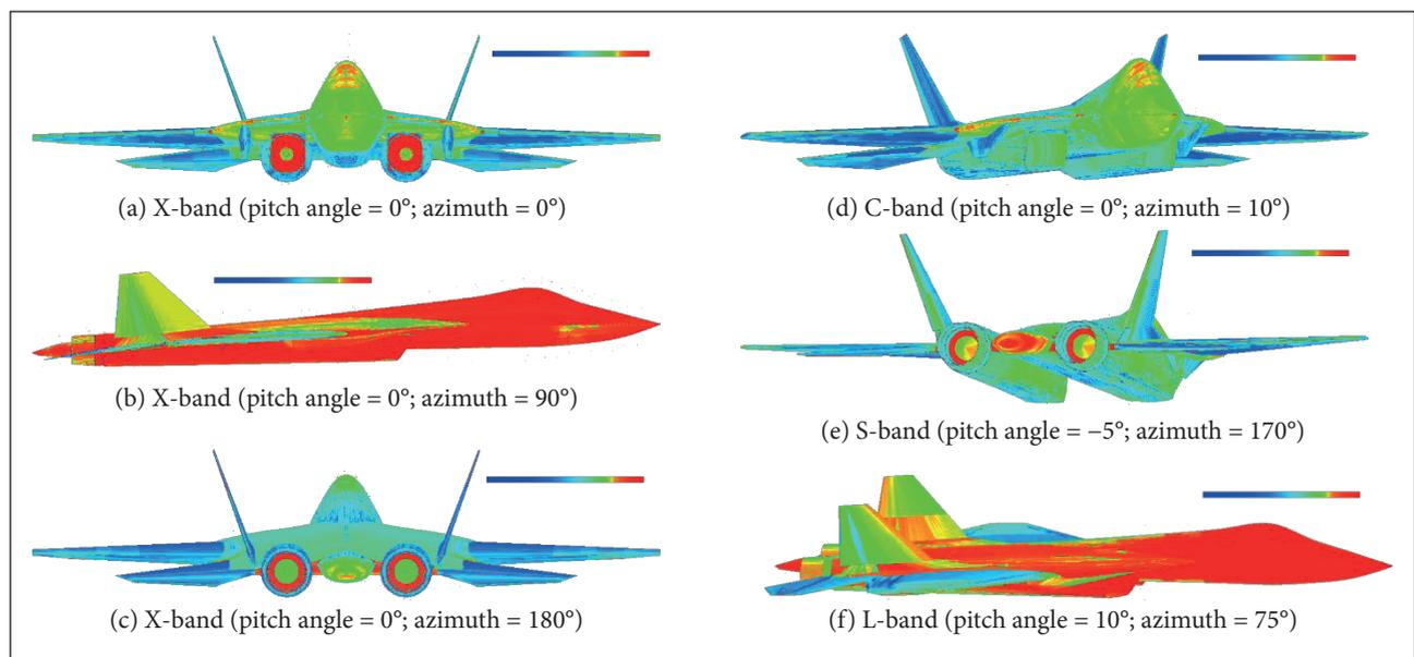
**Figure 4.** RCS scattering properties of aircraft components.
