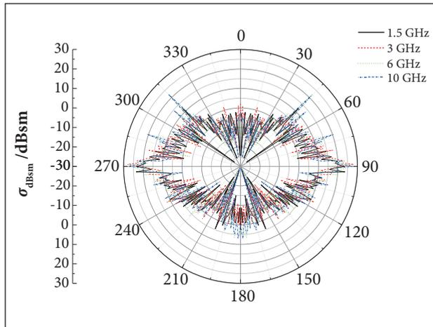
**Figure 3.** RCS characteristic curves (H-H polarization, pitch angle = 0°).
