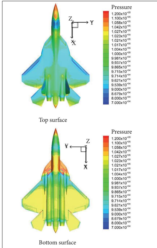
**Figure 6.** Pressure distribution of the conceptual strike-fighter.
