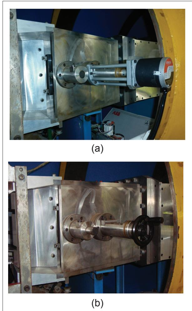
Figure 6. Re-entry flap actuation: (a) modified to remote control actuation, (b) original manual control.
