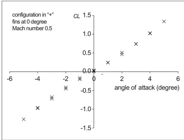
Figure 11. *CL* for configuration in “+”, fins at 0 degree of deflection, Mach number 0.5, and stagnation pressure of 94 kPa.
