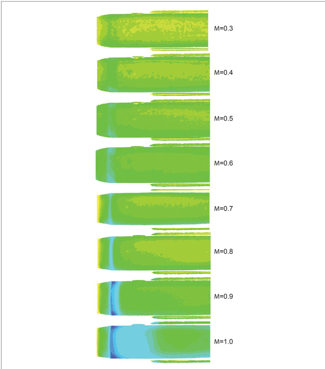
Figure 19. Images obtained with PSP technique showing pressure distribution over the model front region surface, at Mach number from 0.3 to 1.0 and angle of attack at 0 degree.
