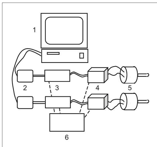
Figure 7. Electronic logical data transference for stepper motor control using PIC.
