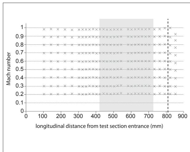
Figure 5. Distribution of the Mach number centerline (shaded area marks the nominal test section region).
