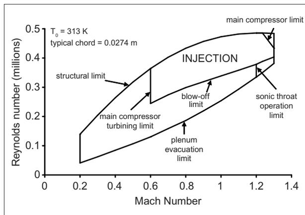
Figure 1. The operational envelope of the TTP.
