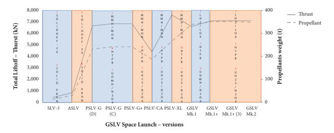
Figure 20. Thrust evolution and propellant types by engine, Space Launch GSLV family.
