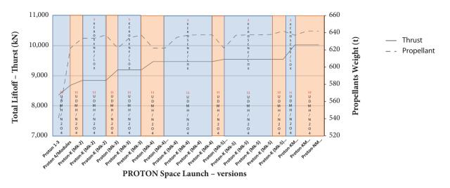
Figure 18. Thrust evolution and propellant types by engine, Space Launch Proton family.
