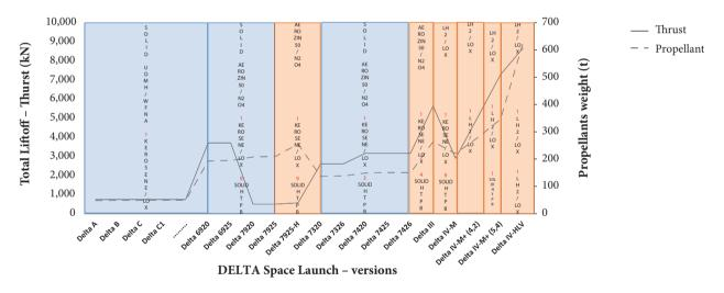
Figure 17. Thrust evolution and propellant types by engine, Space Launch Delta family.
