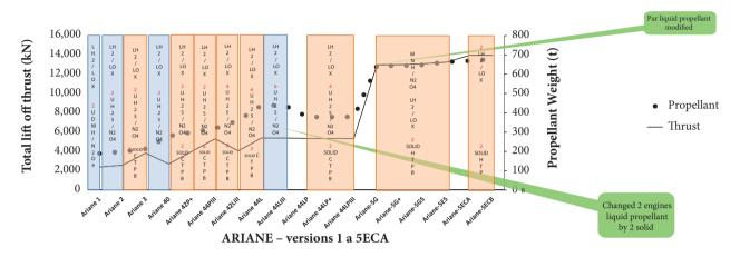
Figure 15. Thrust evolution and propellant types by engine, Space Launch Ariane family.
