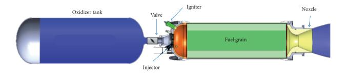
Figure 6. Hybrid engine (credit to Jonny Dyer to SPA... 2014).
