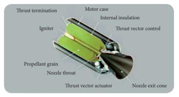
Figure 3. Solid rocket engine (SPA... 2014).
