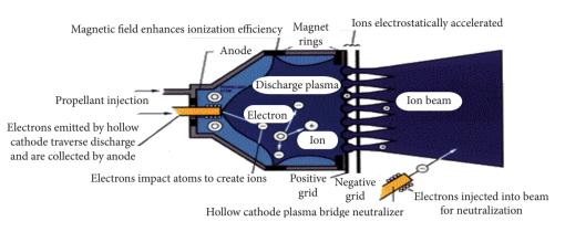
Figure 7. Plasma propulsion engine (NASA 2008).
