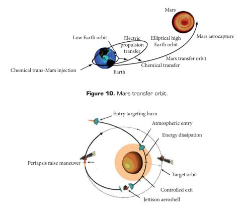
Figure 11. Aerocapture maneuver (Anderson et al. 2010).
