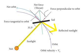
Figure 8. Solar sail propulsion (Johnson et al. 2011).
