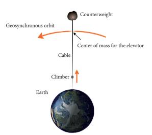
Figure 21. Space elevator concept (EUSpec: 2013).
