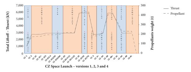
Figure 19. Thrust evolution and propellant types by engine, Space Launch CZ family.
