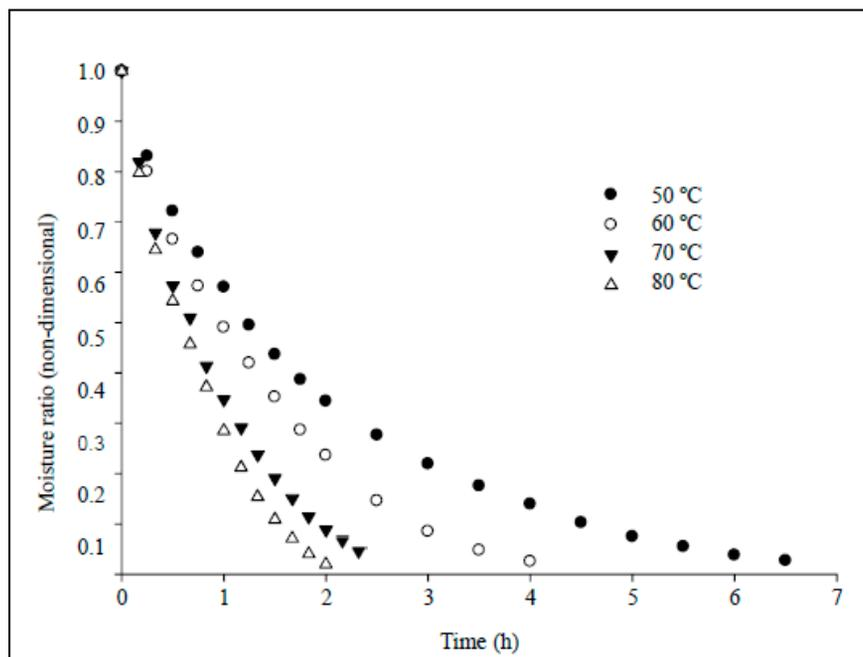
Figure 1. Moisture ratio of endive leaves during drying at 50, 60, 70 and 80°C. Rio Verde, IF Goiano, 2020.
