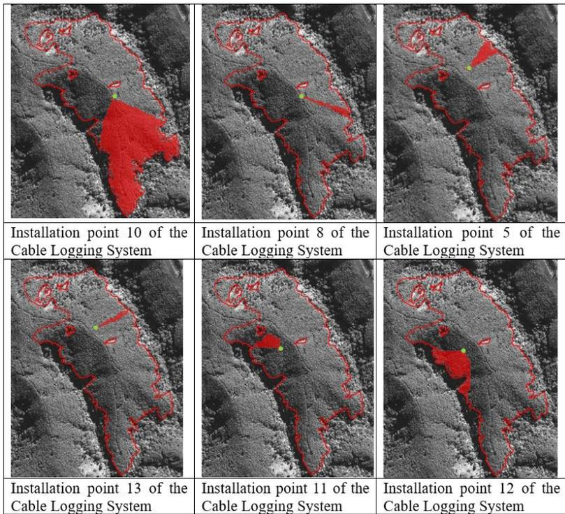
**Figure 3.** Simulation of the optimal cable logging system installation in the scenario for minimizing distance extraction and their respective coverage area (red areas).
