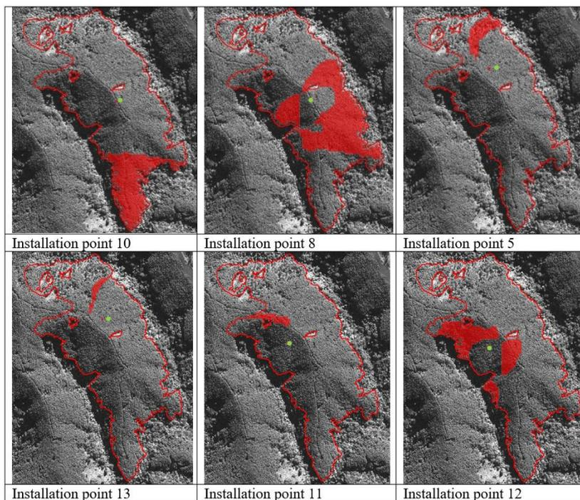
**Figure 2.** Optimum installation simulation of the cable logging system (green points) in the scenario to minimize the operational cycle time of extraction and their coverage areas (red areas).
