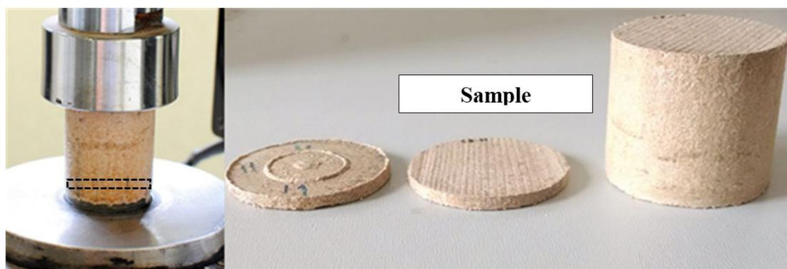
**Figure 2.** Briquette and region from where the samples for X-ray densitometry were obtained.
