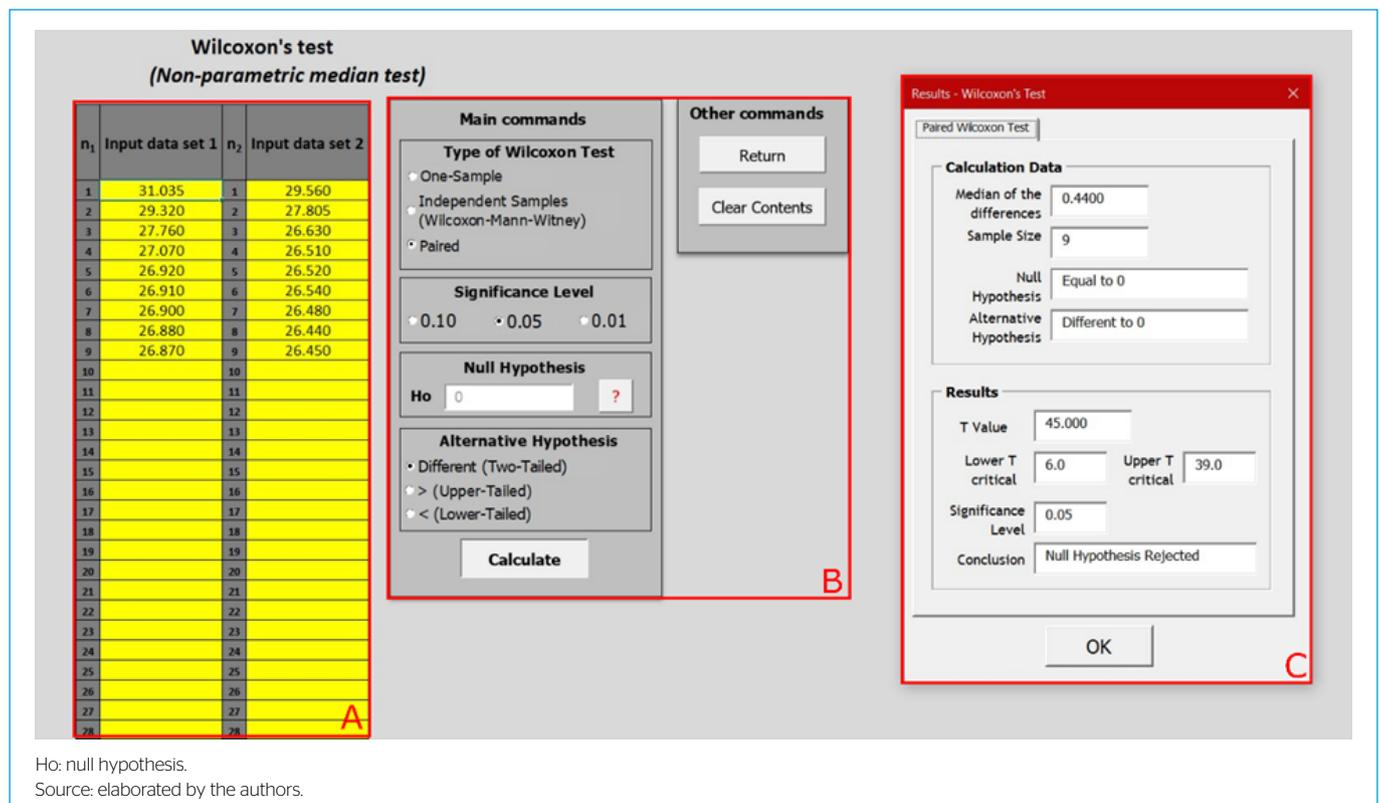
**Figure 9** – Paired Wilcoxon’s test applied to compare the medians of temperatures from different profiles of the Mogi-Guaçu reservoir: (A) input data area; (B) panel control area; (C) output data window.
