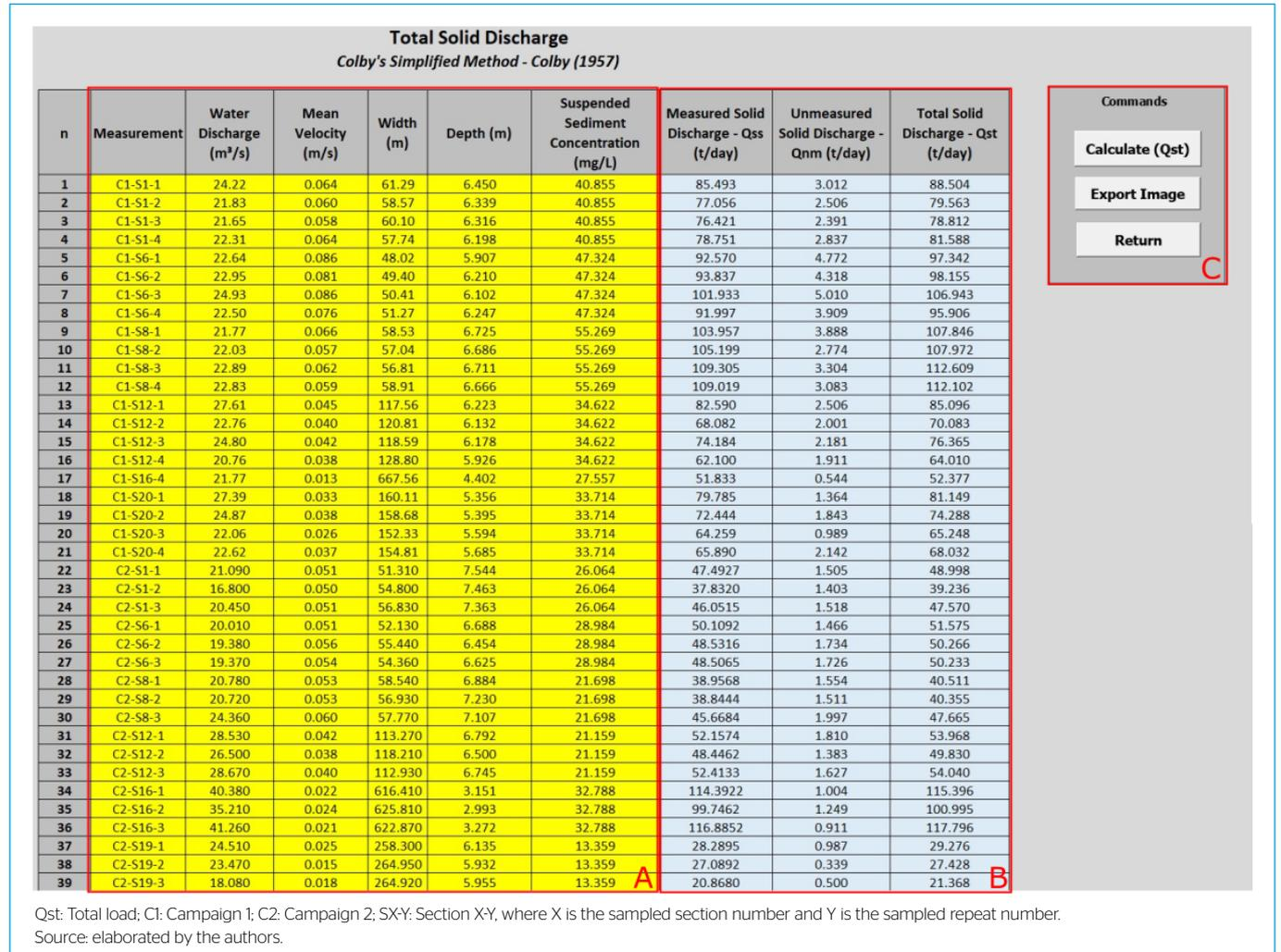
**Figure 3** – Total load calculation screen on NH SEDIMENT AND STATISTIC: (A) input data area for total solid discharge calculation; (B) output data area of measured and unmeasured solid discharge, and total solid discharge; (C) panel control area.
