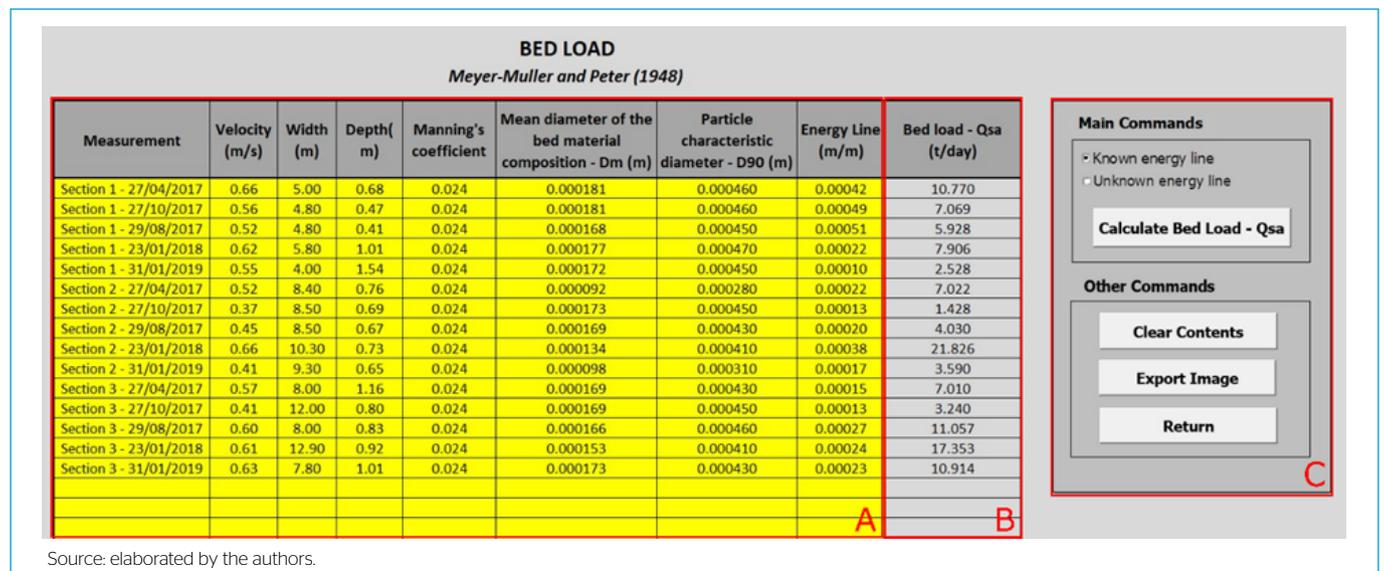
**Figure 4** – Bed load calculation screen on NH SEDIMENT AND STATISTIC: (A) input data area for bed load calculation; (B) output data area; (C) panel control area.
