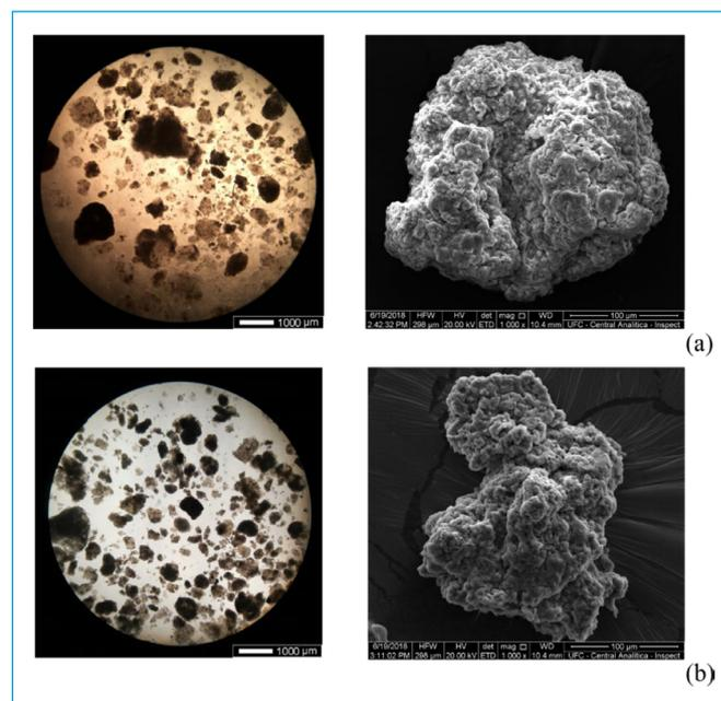
**Figure 2** – Optical and scanning electron microscopy (SEM) micrographs, respectively, of the granules of simultaneous fill/draw SBR in the (A) absence (R1, control) and (B) presence (R2) of coal ash.
