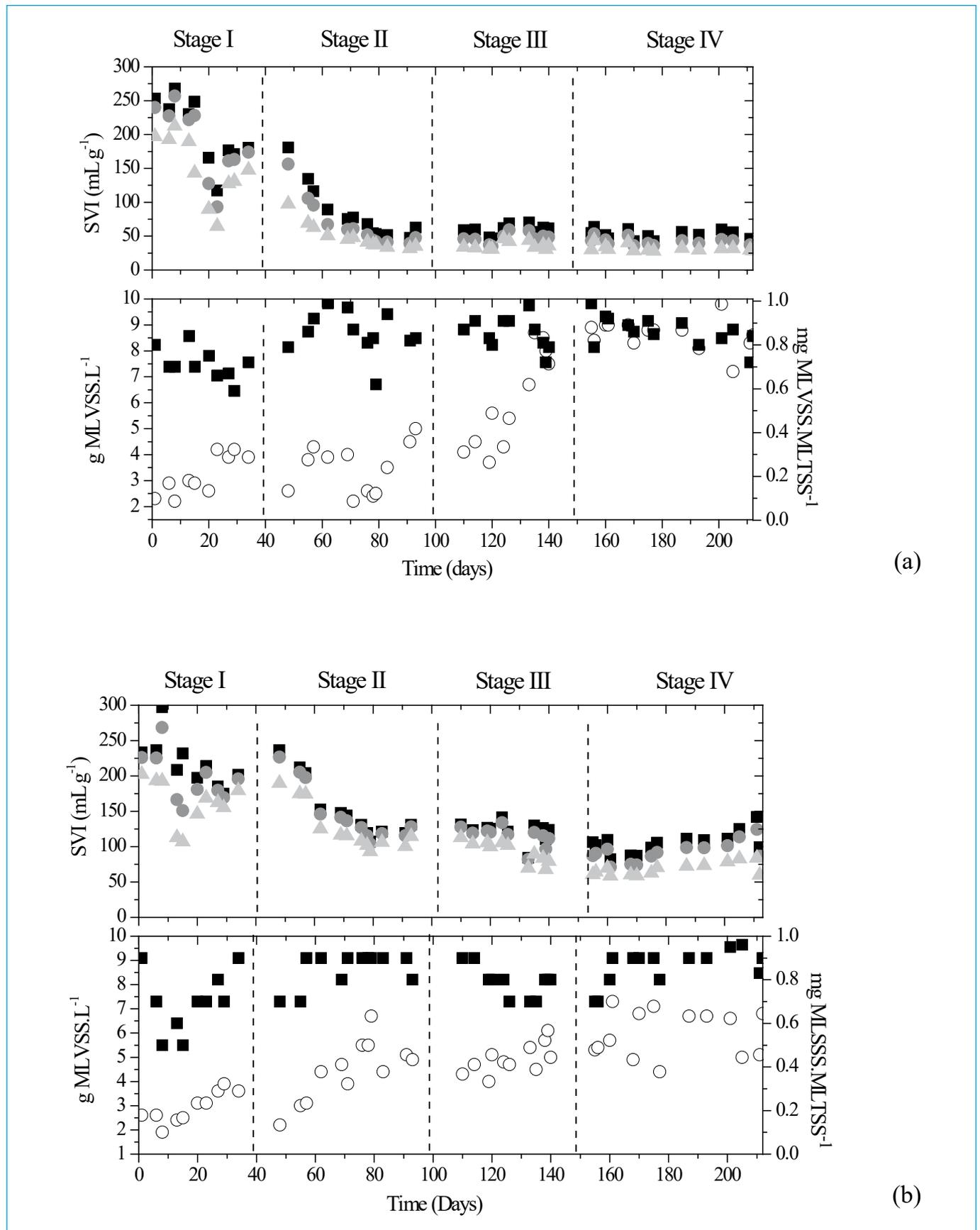
**Figure 1** - Sludge volumetric index and mixed liquor volatile suspended solids values for simultaneous fill/draw SBR operated in the (A) absence (R1, control) and (B) presence (R2) of coal ash (■) SVI<sub>15'</sub>, (●) SVI<sub>10'</sub>, (▲) SVI<sub>30'</sub>, (○) MLVSS and (■) MLVSS/MLSS.
