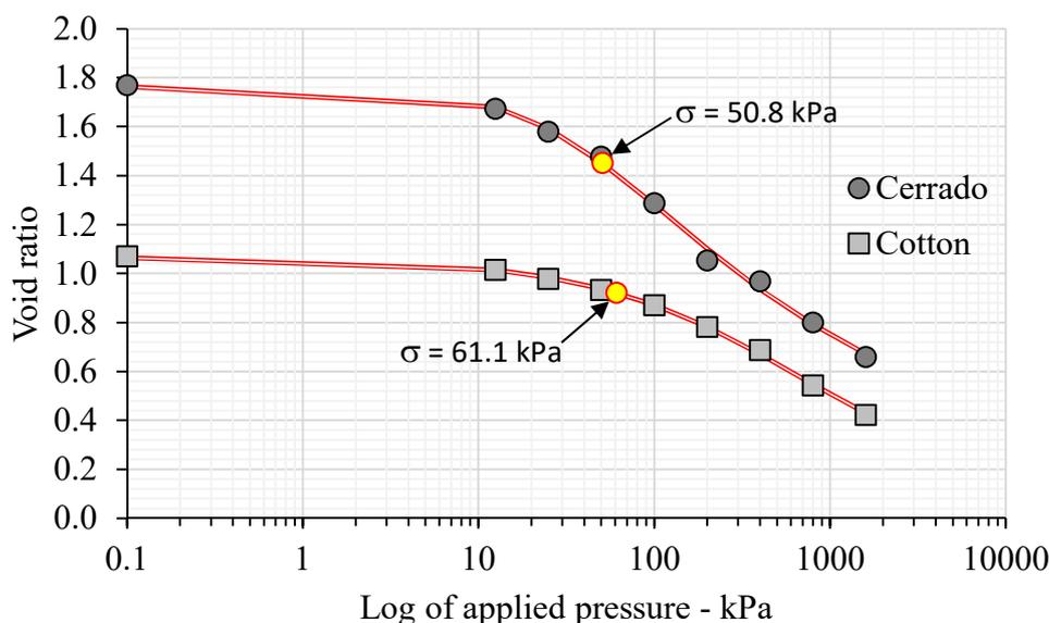
FIGURE 4. Compression curve for Oxisol under native Cerrado and under cotton crop. Pre-consolidation pressure determined by the method of Casagrande (1936) using a plugin implemented in Microsoft Excel (Gubiani et al., 2017).
