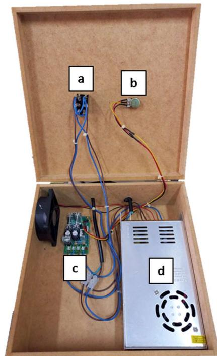
FIGURE 2. Control panel of low-cost electro-mechanical press. a: three position 6-terminal toggle switch; b: potentiometer; c: 12V 30A DC Motor Speed Controller; d: DC 12V power supply.
