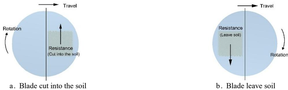
FIGURE 3. Vertical resistance schematic.
