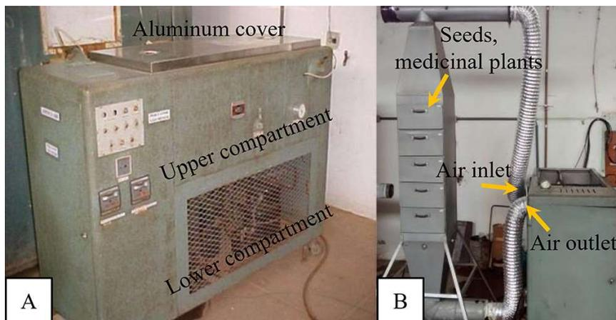
FIGURE 1. Overview of the Aminco-Aire conditioner compartments.
