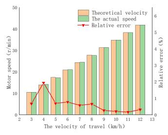
FIGURE 12. Detection of fuzzy PID speed accuracy.
