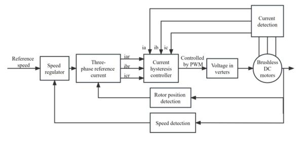
FIGURE 4. Diagram representing the dual closed-loop fuzzy PID control strategy.
