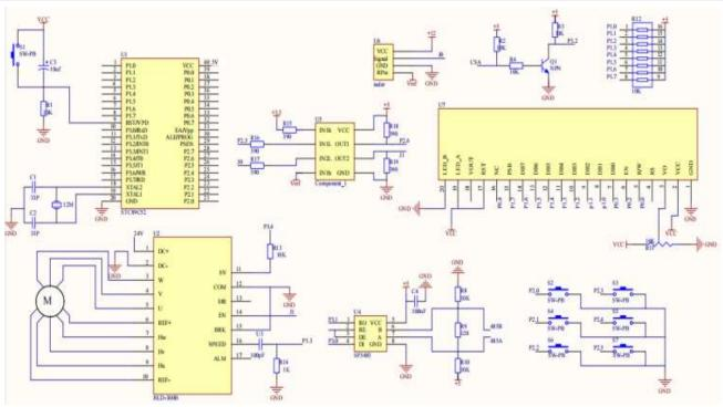
FIGURE 9. Circuitry of microcontrollers.
