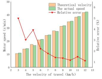
FIGURE 11. Traditional PID speed accuracy detection.
