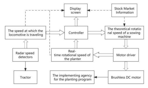
FIGURE 1. Block diagram of the electronic control system.
