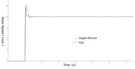
FIGURE 3. Comparison of simulation results (Z-N, PSO).
