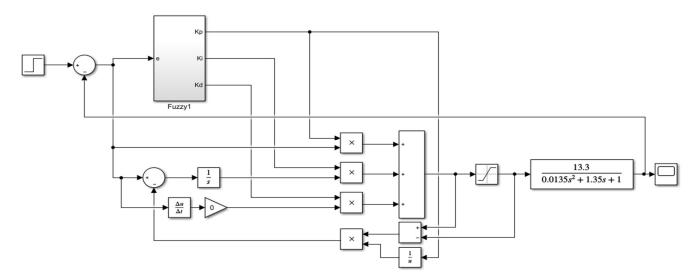
FIGURE 5. Simulation diagram of the fuzzy PID control model for a brushless DC motor.
