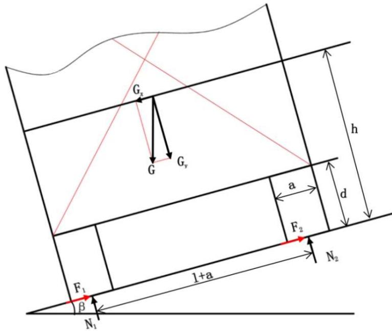
FIGURE 3. Analysis on the force of corn harvested on the slope.
