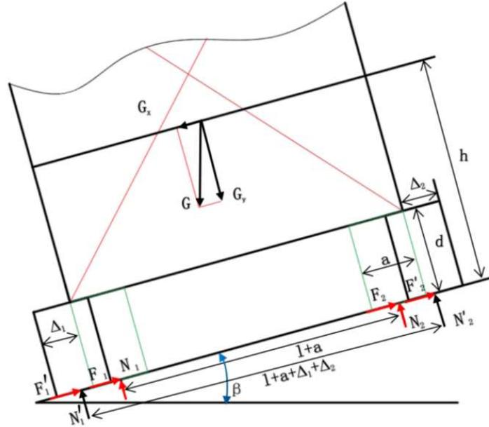
FIGURE 4. Load-bearing analysis after the driving wheel is extended.
