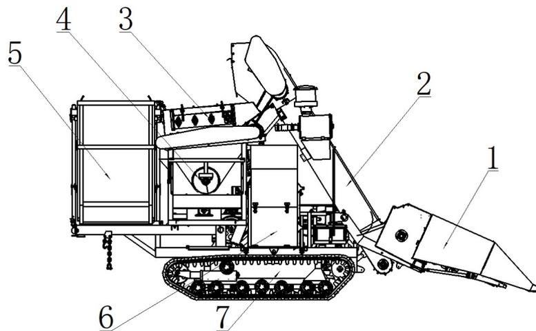
(1) Header (2) Ear lifter (3) Peeling device (4) Grain recovery device (5) Ear collection box (6) Powertrain (7) Wheel spacing adjustable chassis
