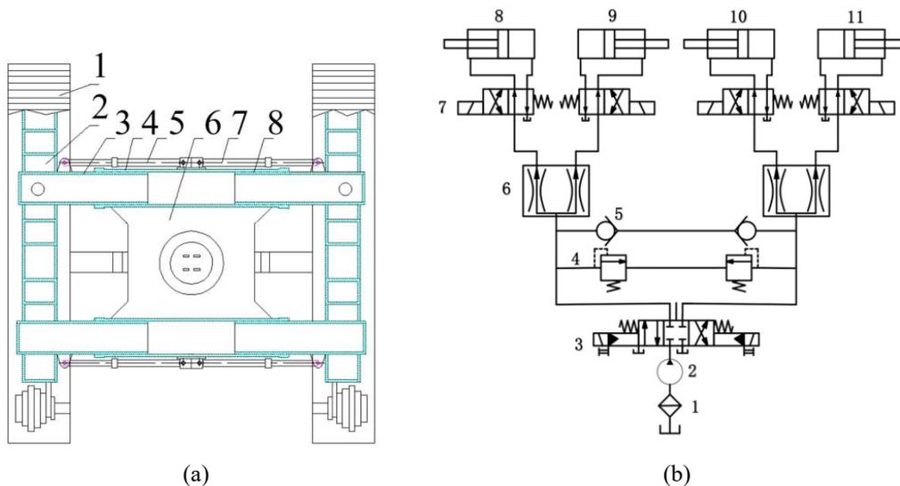
(a) (1) track (2) Left walking beam (3) left telescopic frame (4) fixed frame (5) left telescopic cylinder (6) chassis base (7) right telescopic cylinder (8) right telescopic frame
