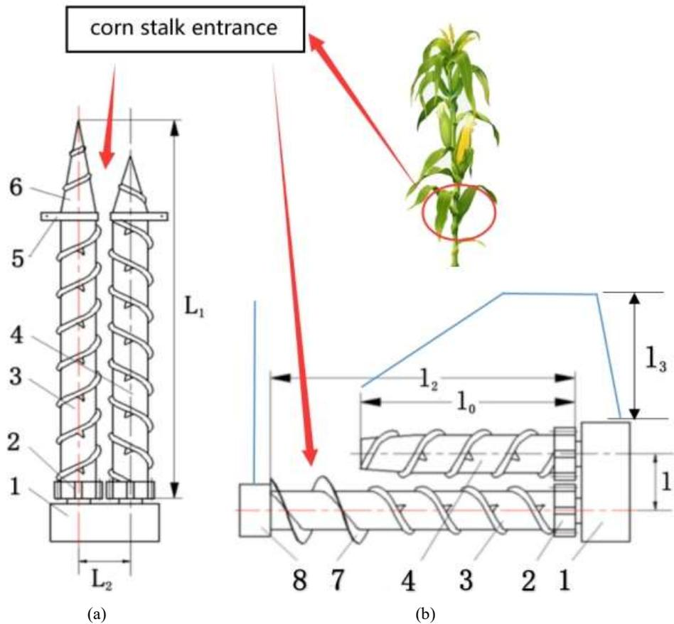
(1) Gearbox (2) Strong pull section (3) Ear picking section (4) Short picking roller (5) Gap adjustment mechanism (6) Guide cone section (7) Leading blade (8) Front bearing seat
