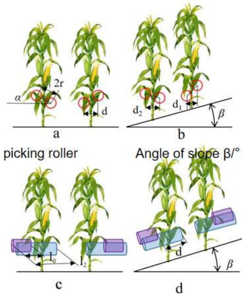
(a) Schematic diagram of the longitudinal roller picking structure for level ground operation
