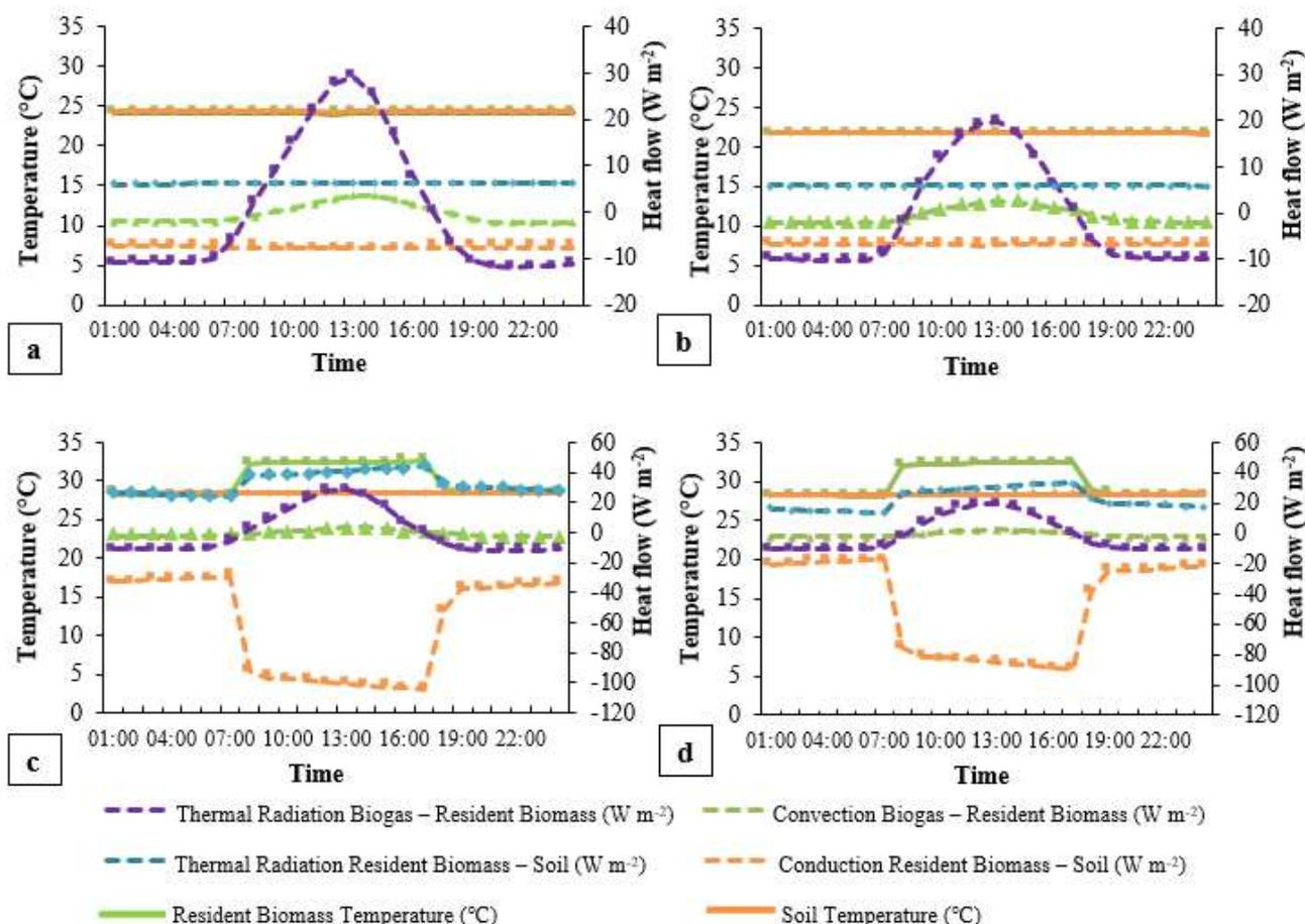
FIGURE 5. Temperature variation for resident biomass and soil, and heat flows ( $q_2$  and  $q_3$ ), from hourly averages for hot (a) and cold (b) periods in the scenario without heating, and hot (c) and cold (d) periods in the scenario with heating.
