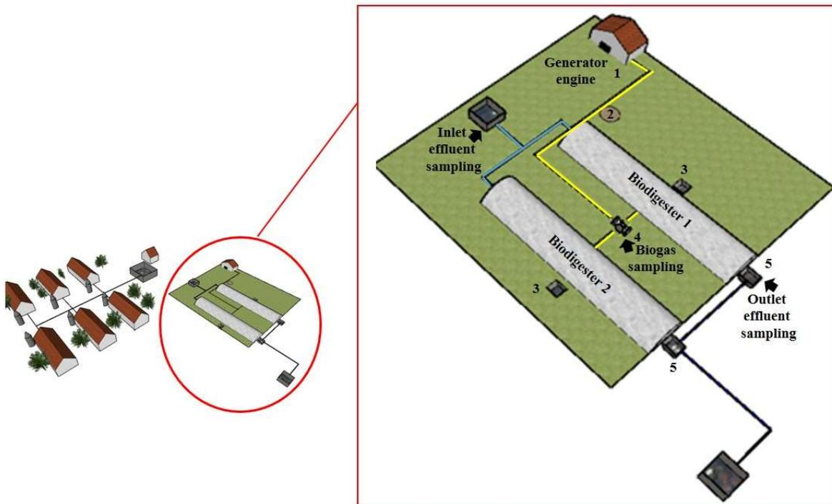
FIGURE 2. Schematic diagram of the effluent treatment station and location sites of the temperature sensors. Source: Sousa et al. (2022). Temperature sensors: 1- Environment, 2- Soil, 3- Resident biomass, 4- Biogas, 5- Digestate
