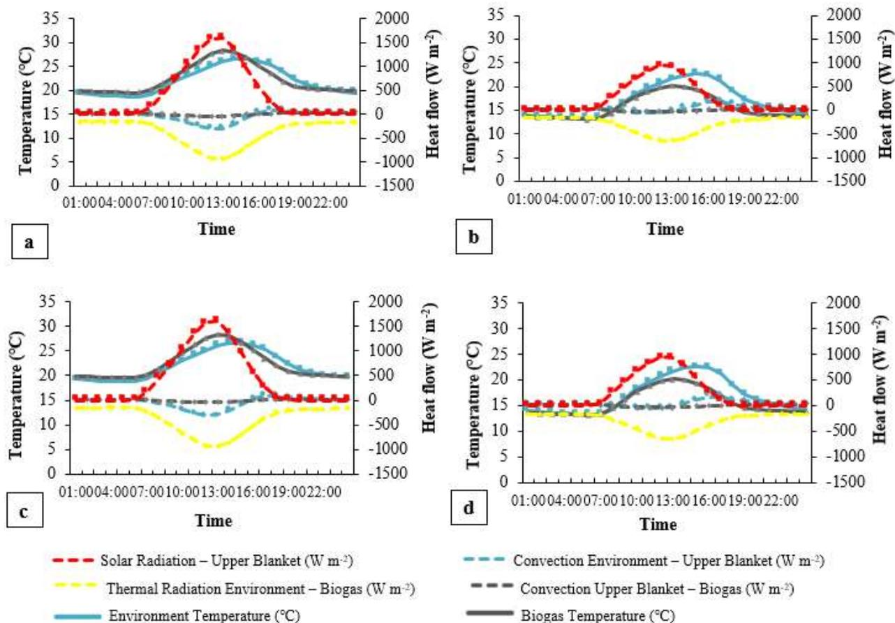
FIGURE 4. Variation in temperature of the environment and biogas, and heat flow ( $q_1$ ) from hourly averages for hot (a) and cold (b) periods in the scenario without heating and for hot (c) and cold (d) periods in the scenario with heating.
