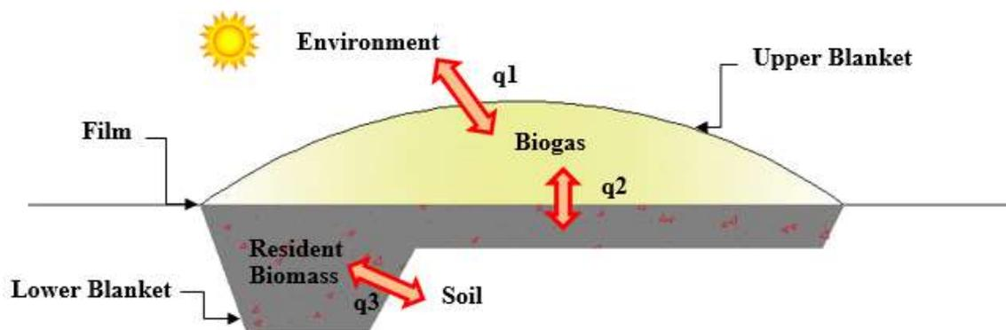
FIGURE 3. Schematic diagram of the thermal exchanges among biodigester, external environment, and soil.
