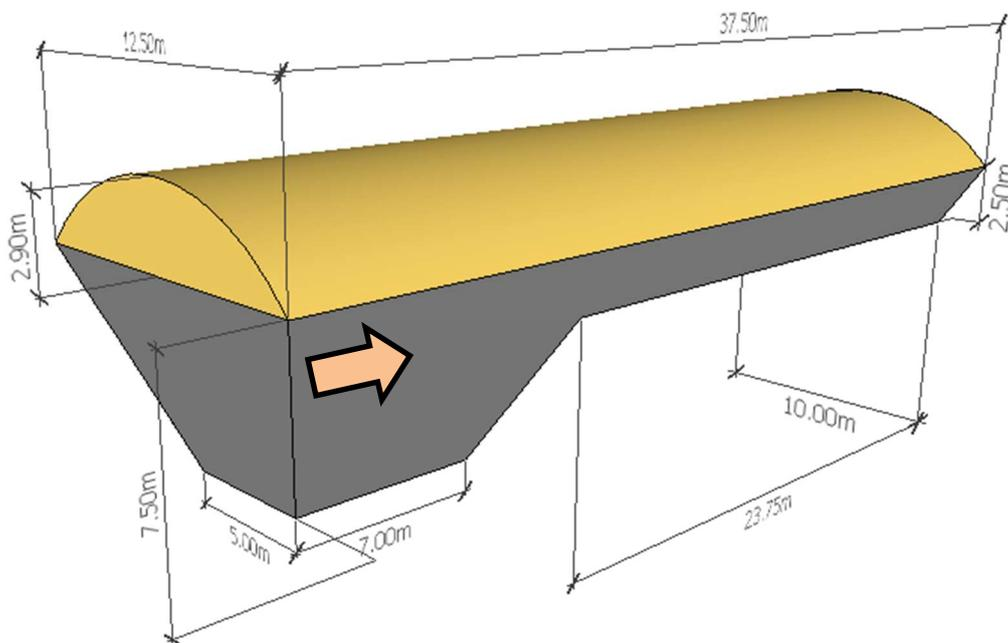
FIGURE 1. Details of the internal and external dimensions of the biodigesters.
