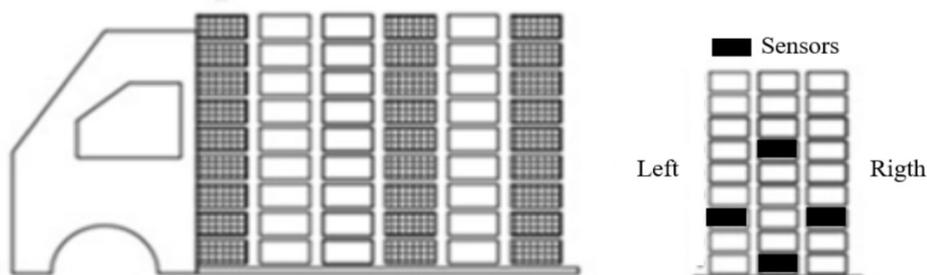
FIGURE 3. Sensor distribution in wind tunnel tests.
