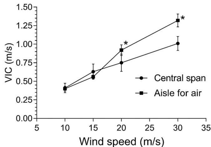
FIGURE 7. Variation of ventilation inside the crates (VIC)  $\pm$  standard mean error as a function of the test speed in the wind tunnel in the evaluated layouts.
