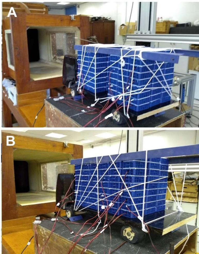
FIGURE 2. Representation of wind tunnel tests with truck prototypes using a “central span” (A) and air corridor (B) layout
