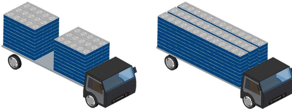
FIGURE 1. Virtual models: layout with central span (A) and with air aisle (B).
