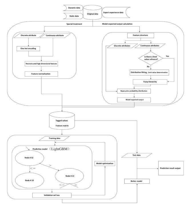
Figure 2. Flow chart of the algorithm using LightGBM.
