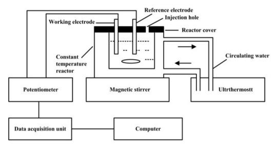
Figure 1. Schematic diagram of nonlinear chemical oscillation system.
