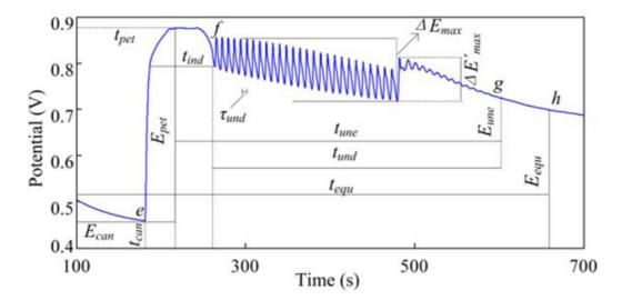
Figure 2. Basic characteristic information of oscillation spectrum of milk powder. e-f: inductive curve; f-g: fluctuation curve; g-h: stop wave curve; point e and h are the start point and end point of reaction, respectively.
