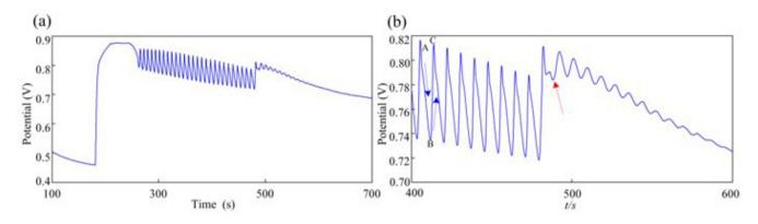
Figure 3. Interference of  $1 \times 10^{-1}$  mol/L potassium iodide solution on oscillation spectrum of milk powder. (a) Integral graphic, (b) Corresponding local graphic.
