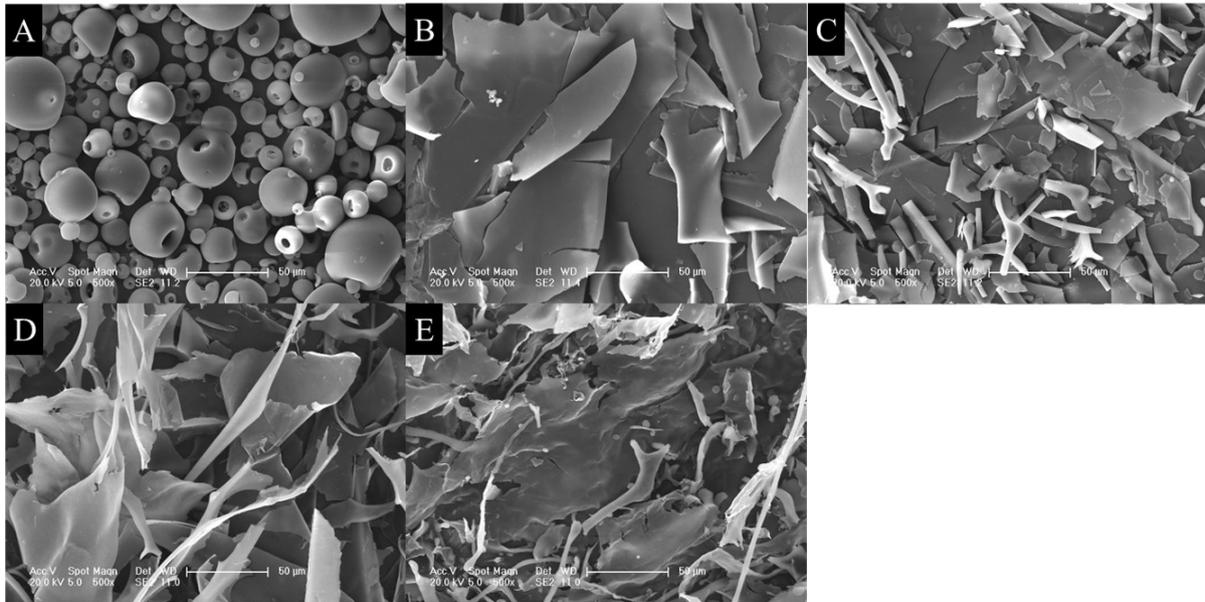
**Figure 5.** SEM images of OVA (A), H-OVA (B), U-OVA (C), HG-OVA (D), UG-OVA (E) (Magnification: 500×). OVA, native ovalbumin; H-OVA, ovalbumin solution treated by heating (90 °C for 50 min) in water bath; U-OVA, ovalbumin solution treated by ultrasound (500 W for 70 min at 60 °C); HG-OVA, the mixture of ovalbumin and pectin treated by heating at 90 °C for 50 min; UG-OVA, the mixture of ovalbumin and pectin treated by the high-intensity ultrasound at the power of 500 W for 70 min at 60 °C.
