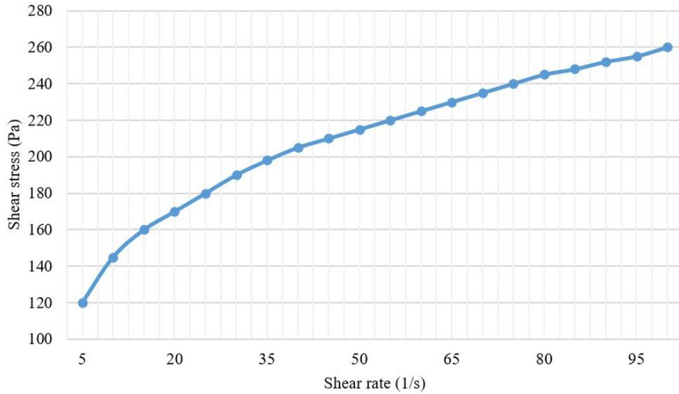
Figure 2. Dependence of the shear stress and the shear rate of mayonnaise with acacia honey (10,000 rpm, 2 min) at 25 °C.
