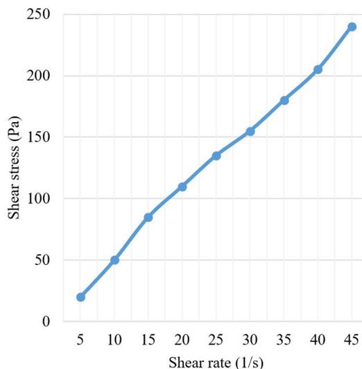
**Figure 1.** The relationship between the shear stress and the shear rate of spring honey at 25 °C.
