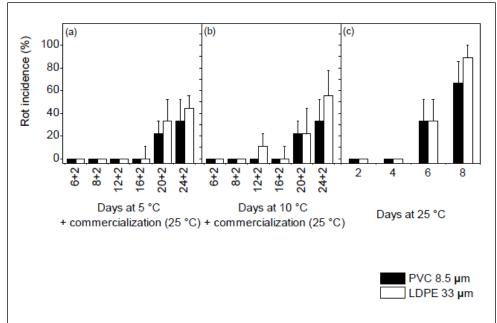
Figure 5 - Rot incidence (%) of 'Malasia' star fruit packed in polystyrene trays covered with polyvinyl chloride - PVC (8.5  $\mu$ m thick) and low-density polyethylene - LDPE (33  $\mu$ m thick) and stored for eight days at 25±1 °C / 85 ± 5% RH (c) and for up to 24 days at 10±1 °C (b) and 5±1 °C (a), followed by two days at 25±1 °C / 85 ± 5% RH. Vertical bars indicate mean standard error (n=3).
