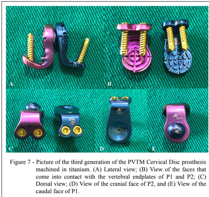
Figure 7 - Picture of the third generation of the PVTM Cervical Disc prosthesis machined in titanium. (A) Lateral view; (B) View of the faces that come into contact with the vertebral endplates of P1 and P2; (C) Dorsal view; (D) View of the cranial face of P2, and (E) View of the caudal face of P1.
