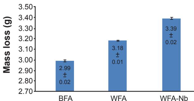
Figure 3: Results of mass loss of AISI D2 steel specimen after abrasiveness trials with brown fused alumina (BFA), white fused alumina (WFA), and white fused alumina with niobium oxide (WFA-Nb).
