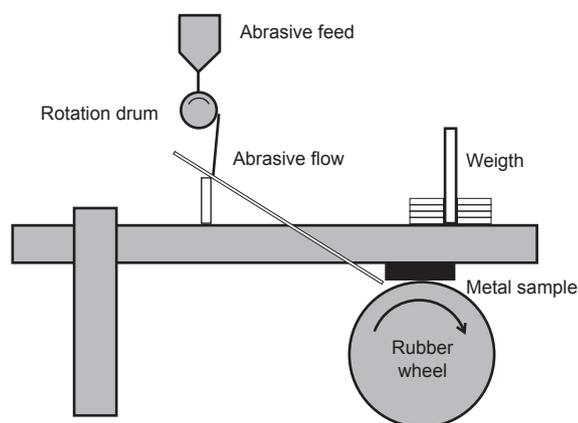
Figure 2: Layout drawing of horizontal rubber wheel equipment.
