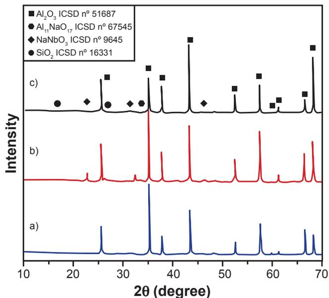
Figure 4: XRD patterns of the samples of grits of: a) brown fused alumina (BFA); b) white fused alumina with niobium oxide (WFA-Nb); and c) white fused alumina (WFA).
