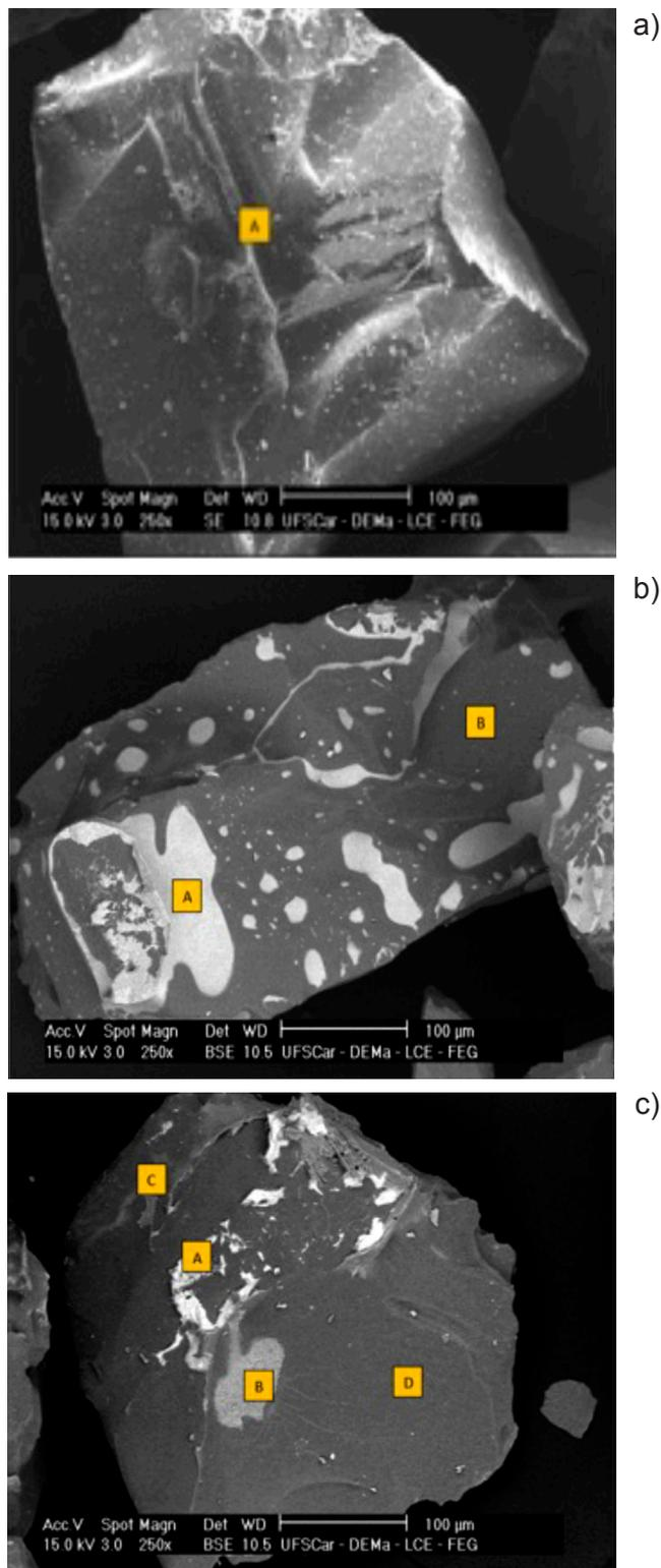
Figure 5: SEM micrographs of P60 grits of: a) white fused alumina (WFA); b) white fused alumina with the addition of niobium oxide (WFA-Nb); and c) brown aluminum oxide (BFA).
