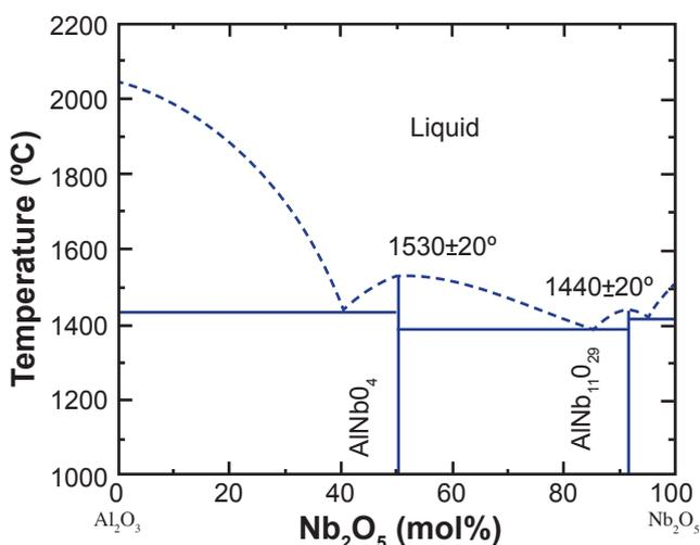
Figure 1: Equilibrium phase diagram of  $\text{Al}_2\text{O}_3\text{-Nb}_2\text{O}_5$  [10].
