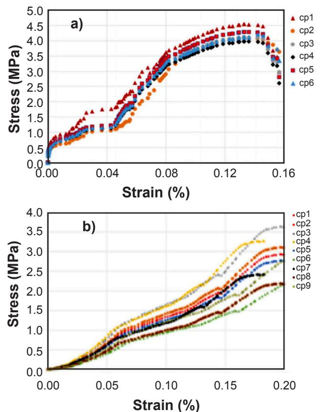
Figure 2: Stress-strain curves for the studied blocks (a) and mortars (b).
