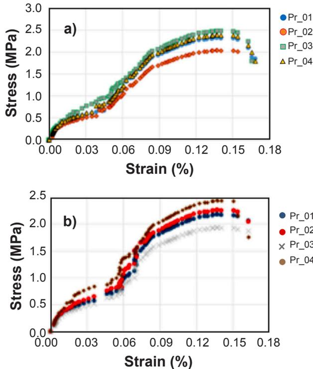
Figure 3: Stress-strain curves for prisms without (a) and with (b) mortar.
