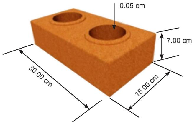
Figure 1: Illustration of the plug-in block used.
