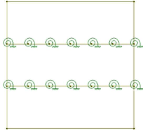
Figure 4: Representation of a prism with mortars functioning as elastic support.
