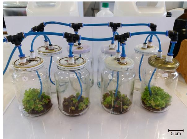
**Figure 1:** Bioreactor with dual container system (500 mL capacity).
