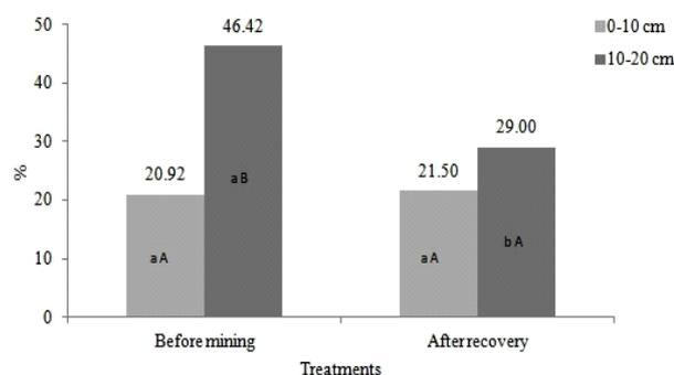
Figure 1 – Stoniness index values for soils collected at different depths before mining intervention and after the environmental recovery of bauxite deposits in the plateau region in Poços de Caldas, Minas Gerais, Brazil.
