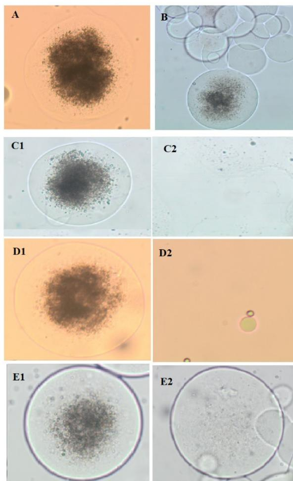
**Figure 1:** Microscopic images of the microcapsules in contact with different aqueous media: (A) 1.5 M ionic strength; (B) 4 °C after agglomeration; (C1 and C2) 30 °C before and after disintegration, respectively; (D1 and D2) pH 3.8 before and after disintegration, respectively; (E1 and E2) Oil released through microcapsules, after 1 and 7 hours, respectively.
