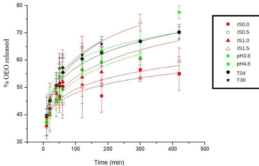
**Figure 2:** OEO release profiles in different aqueous media and solid curves representing the fitted Peppas model.
