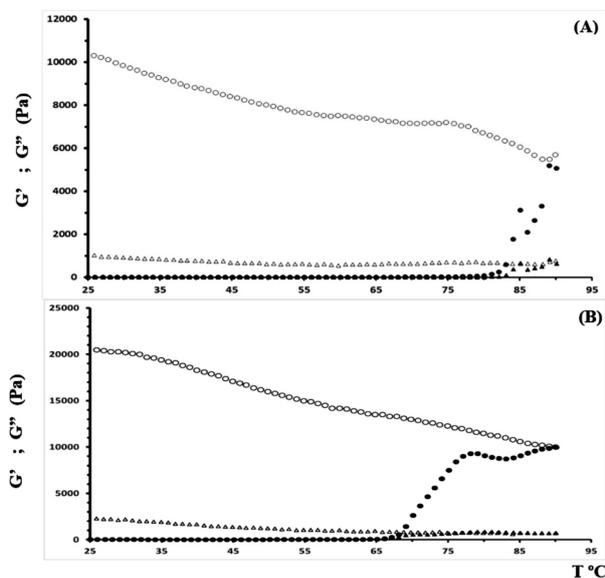
**Figure 2.** Dependence of elastic modulus ( $G'$ ) and viscous ( $G''$ ) with respect to temperature in the albumen (A) and yolk (B). Heating ( $\bullet G'$ ;  $\blacktriangle G''$ ). Cooling ( $\circ G'$ ;  $\triangle G''$ ).
