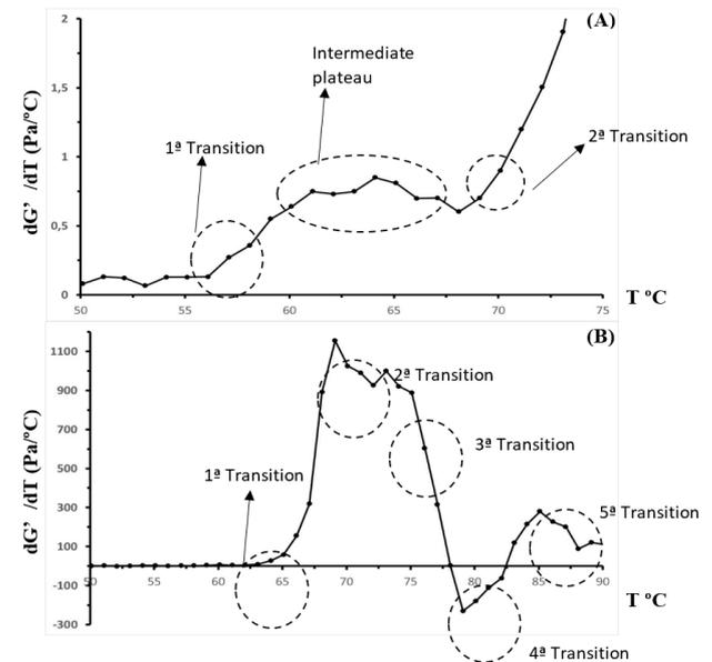
**Figure 3.** Transitions of behavior of the rate of change of the elastic modulus as a function of the heating temperature ( $dG'/dT$ ) throughout the albumen heating (A) and yolk (B) of rhea egg stored for seven days at 10°C
