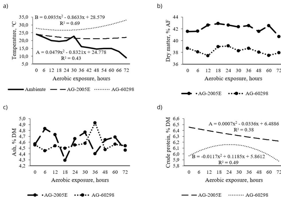
**Figure 2.** Temperature (a), dry matter (b), ash (c), and crude protein (d) of the silages of sorghum hybrids AG-2005E and AG-60298, as a function of different aerobic exposure times
