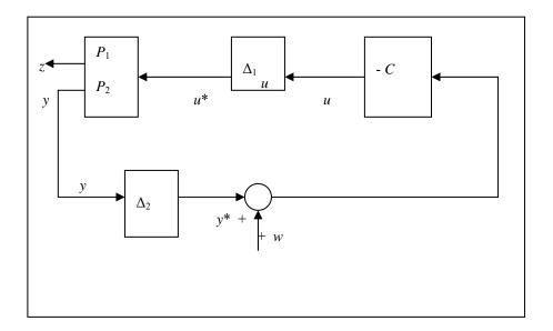
In the block diagram below the inputs and outputs are Laplace-transforms of multivariable signals. w(s) is the Laplace transform of the signal to be asymptotically rejected at the inverse Laplace-transform of z(s).
