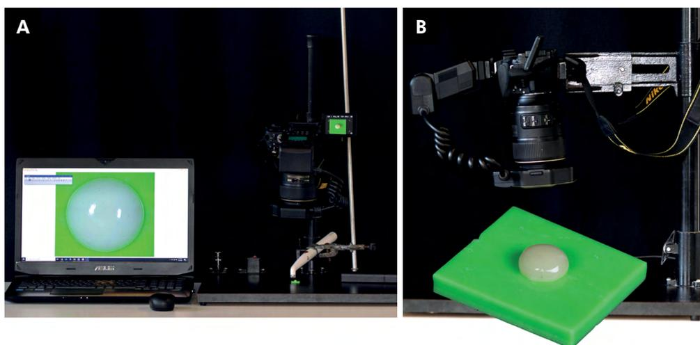
**Figure 1.** Experimental setup of the optical method using a DSLR camera, 105 mm macro lens and a ring flash. Frontal view (A); Side view (B).
