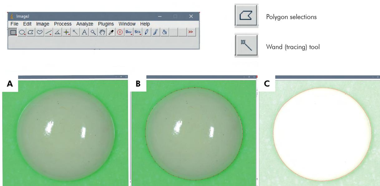
**Figure 2.** Analysis in the image analysis software (Image J) of the pre- and post-polymerization sample. Pre-polymerization image (A); the contours of the samples drawn on the captured images with Polygon Selections tool (B); Brightness adjustment for better outline visualization with the Wand Tool (C).
