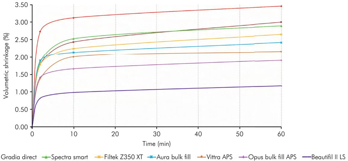
**Figure 3.** Total shrinkage (volume %) for the eight restorative composites against time (0–60 min).
