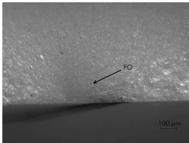
**Figure 3.** Representative image (90x magnification) of the fracture origin (FO) located on the surface of the sample (Group 120A).
