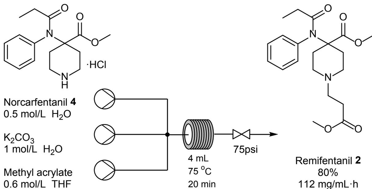
**FIGURE 3** - Continuous flow setup scheme for preparing remifentanyl.
