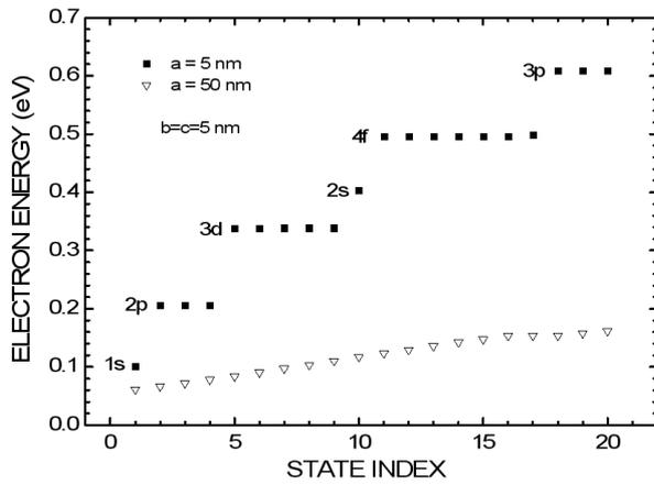
FIG. 1: Electron energy levels of ellipsoidal CdSe QDs as a function of the state index for a changing volume with  $\beta=1$  (squares) and  $\beta=10$  (down triangles). The energy states of spherical QDs are labeled using atomic notation.
