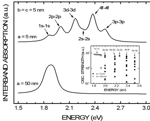
FIG. 2: Interband absorption of spherical ( $a=5$  nm or  $\beta=1$ ) and ellipsoidal ( $a=50$  nm or  $\beta=10$ ) CdSe QDs. In the inset, the oscillator strength is presented for both cases to show the role of each transition.
