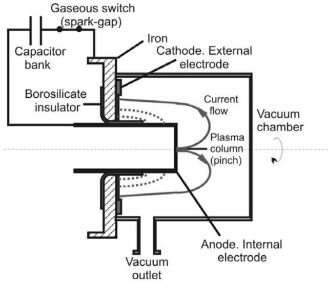
FIG. 1: Diagram of an open-cathode Plasma Focus.
