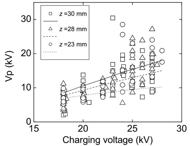
FIG. 5: Peak voltage along the pinch measured and calculated for different charging voltages and different anode lengths.
