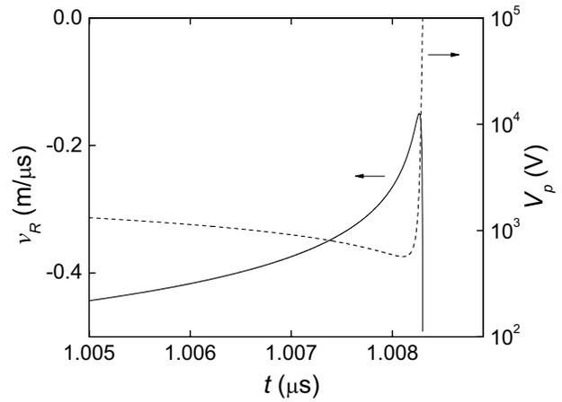
FIG. 4: Numerical evolution of the velocity of the pinch and voltage-drop along the pinch.
