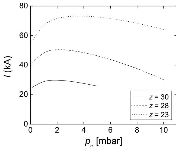
FIG. 7: Charging-pressure dependence of the pinch current calculated for different anode lengths.
