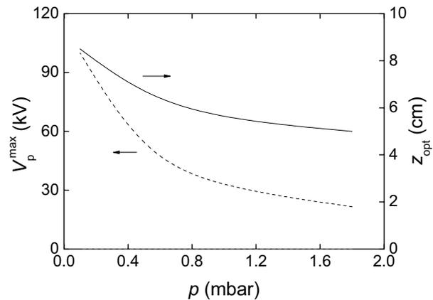
FIG. 9: Optimum pinch voltage and the corresponding optimum anode length.
