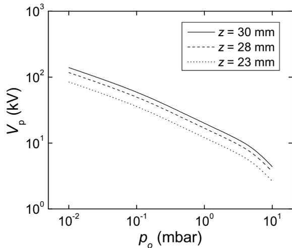
FIG. 6: Charging-pressure dependence of the peak voltage along the pinch calculated for different anode lengths.
