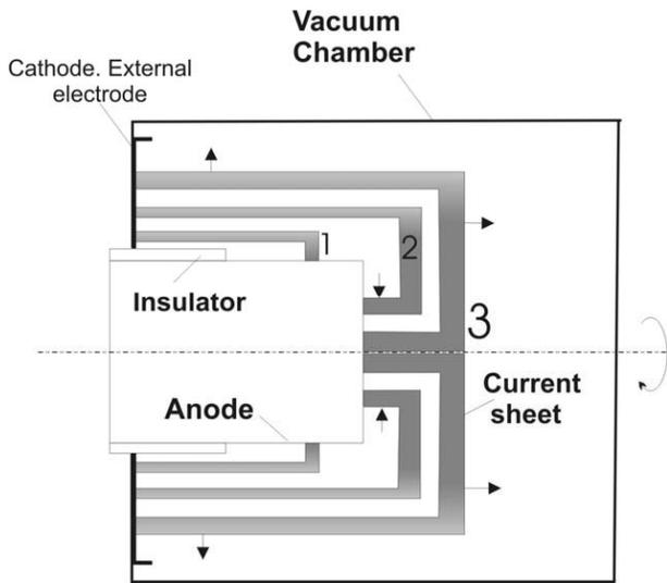
FIG. 2: Lumped parameter model of an open-cathode Plasma Focus (1. Breakdown and run-down, 2. Run-over, 3. Pinch).
