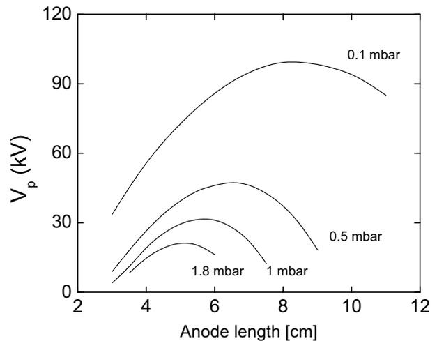
FIG. 8: Peak pinch voltage as function of the anode length.
