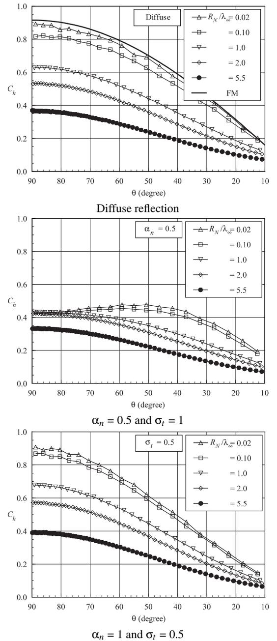
FIG. 5: Distribution of the heat transfer coefficient  $C_h$  along the cylindrically portion of the round leading edges by considering (a) diffuse reflection, (b)  $\alpha_n = 0.5$  and  $\sigma_t = 1$ , and (c)  $\alpha_n = 1$  and  $\sigma_t = 0.5$ .
