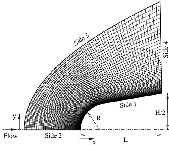
FIG. 3: Schematic view of the computational domain.
