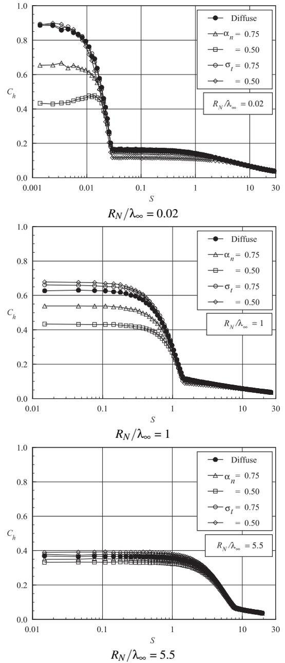
FIG. 4: Distributions of the heat transfer coefficient  $C_h$  along the body surface as a function of the accommodation coefficient for round leading edges with  $R_N/\lambda_\infty$  of (a) 0.02, (b) 1 and (c) 5.5.
