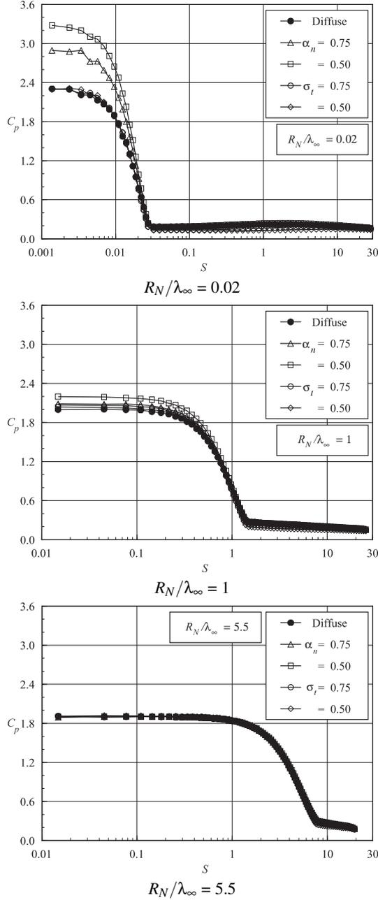
FIG. 7: Distributions of pressure coefficient  $C_p$  along the body surface as a function of the accommodation coefficient for round leading edges with  $R_N/\lambda_\infty$  of (a) 0.02, (b) 1 and (c) 5.5.
