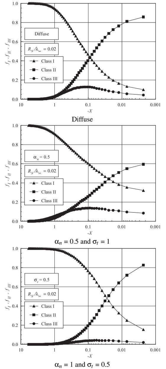
FIG. 10: Distributions of molecules for classes I, II and III along the stagnation streamline for the round leading edge case with  $R_N/\lambda_\infty = 0.02$ : (a) diffuse reflection, (b)  $\alpha_n = 0.5$  and  $\sigma_t = 1$ , and (c)  $\alpha_n = 1$  and  $\sigma_t = 0.5$ .
