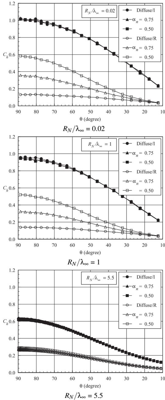
FIG. 6: Distribution of the incident and reflected contributions of the heat transfer coefficient  $C_h$  along the cylindrical portion of the round leading edges with  $R_N/\lambda_\infty$  of (a) 0.02, (b) 1 and (c) 5.5.
