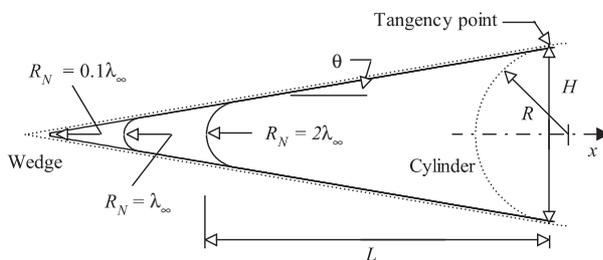
FIG. 2: Drawing illustrating the leading edge geometries.
