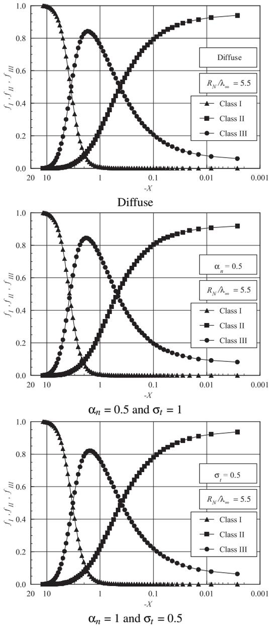
FIG. 11: Distributions of molecules for classes I, II and III along the stagnation streamline for the round leading edge case with  $R_N/\lambda_\infty = 5.5$ : (a) diffuse reflection, (b)  $\alpha_n = 0.5$  and  $\sigma_t = 1$ , and (c)  $\alpha_n = 1$  and  $\sigma_t = 0.5$ .
