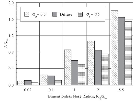
FIG. 12: Dimensionless shock wave standoff distance  $\Delta/\lambda_\infty$  along the stagnation streamline for round leading edges as a function of the normal and tangential accommodation coefficients.
