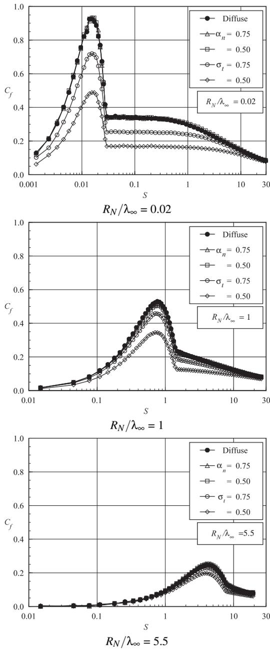
FIG. 8: Distributions of skin friction coefficient  $C_f$  along the body surface as a function of the accommodation coefficient for round leading edges with  $R_N/\lambda_\infty$  of (a) 0.02, (b) 1 and (c) 5.5.
