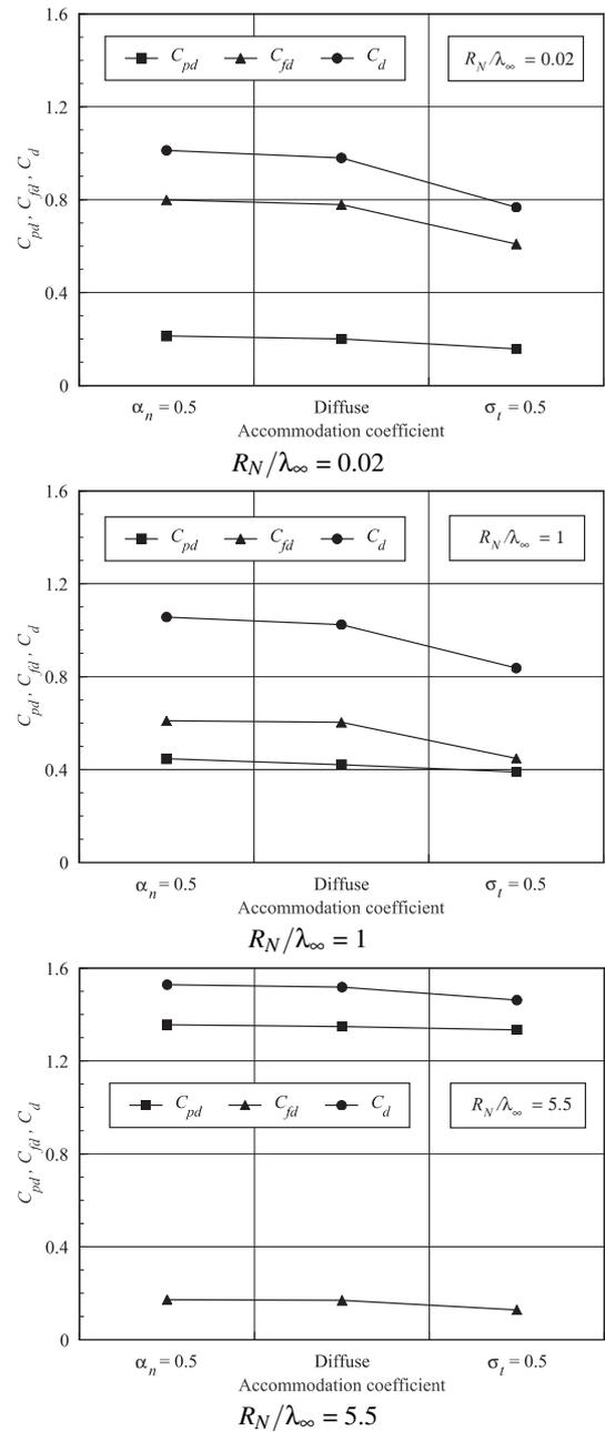
FIG. 9: Pressure drag  $C_{pd}$ , skin friction drag  $C_{fd}$  and total drag coefficient  $C_d$  as a function of the accommodation coefficient for round leading edges with  $R_N/\lambda_\infty$  of (a) 0.02, (b) 1 and (c) 5.5.
