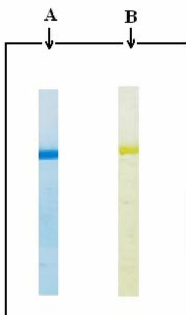
**Figure 4.** NATIVE PAGE of the *Proteus mirabilis* strain ATCC 29245. The purified cytochrome b was run on NATIVE PAGE and stained. Column A: Commassie brilliant blue staining of heme b, Column B: Heme Staining of heme b.
