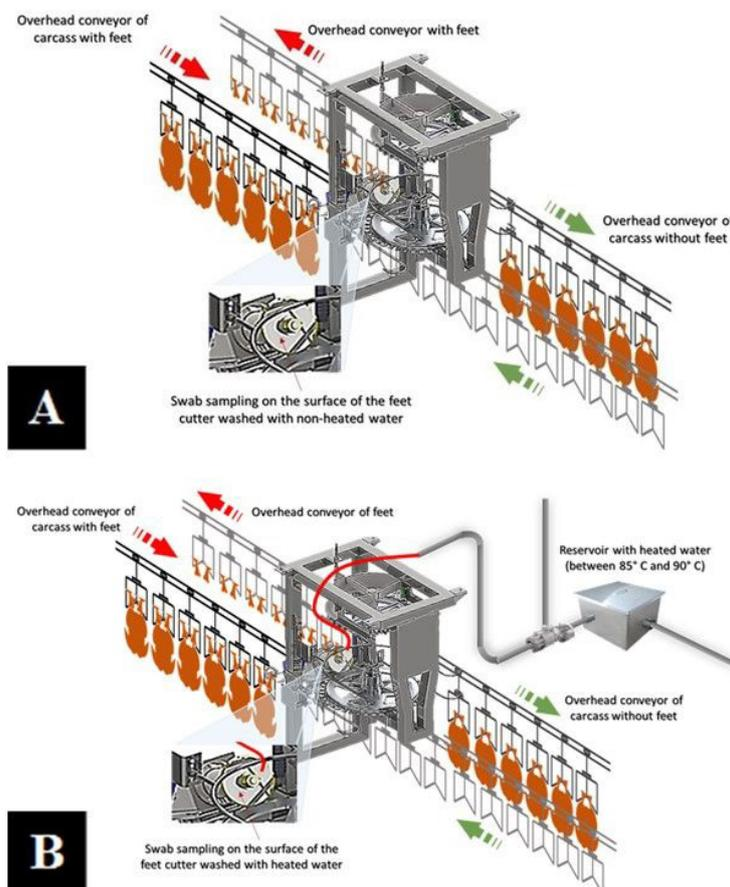
**Figure 1.** Schematic designs of the operational self-washing system of the feet-cutter disc with (A) non-heated and (B) heated water.
