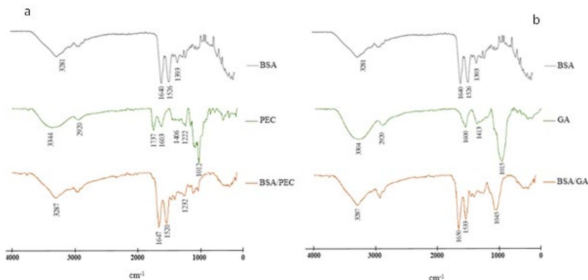
**Figure 5.** FTIR spectra for (a) BSA, PEC and BSA:PEC (10:1) at pH 4.5 without addition of NaCl and (b) BSA, GA and BSA:GA (3:1) at pH 4.0 without addition of NaCl.
