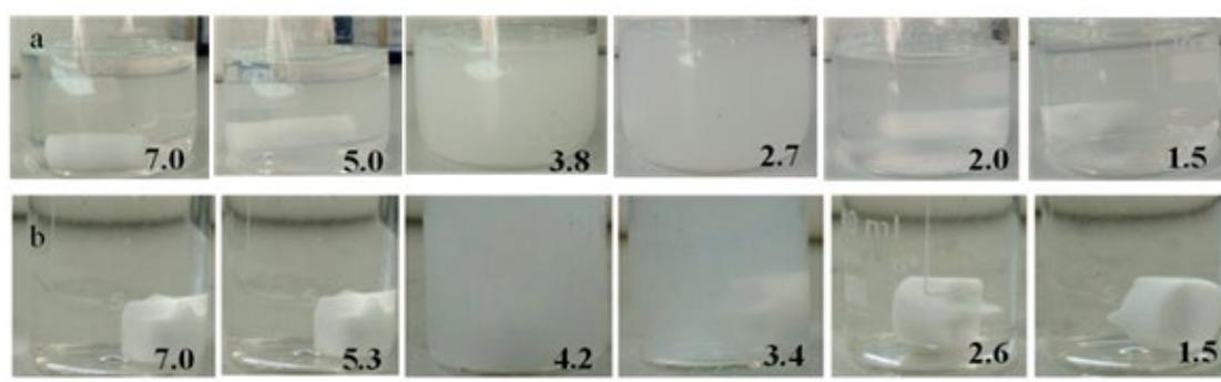
**Figure 2.** (a) Photographs of solutions containing BSA:PEC (10:1) and (b) BSA:GA (3:1) at different pH.
