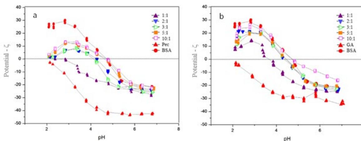
**Figure 3.** pH-dependent potential of the samples containing (a) PEC and BSA:PEC and (b) GA complexes and BSA:GA complexes in different ratios.
