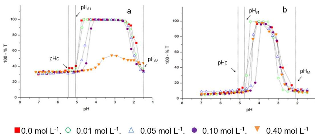
**Figure 4.** Influence of different NaCl concentrations on the turbidity of samples containing (a) BSA:PEC in a ratio of 10:1 and (b) BSA:GA in a ratio of 3:1.
