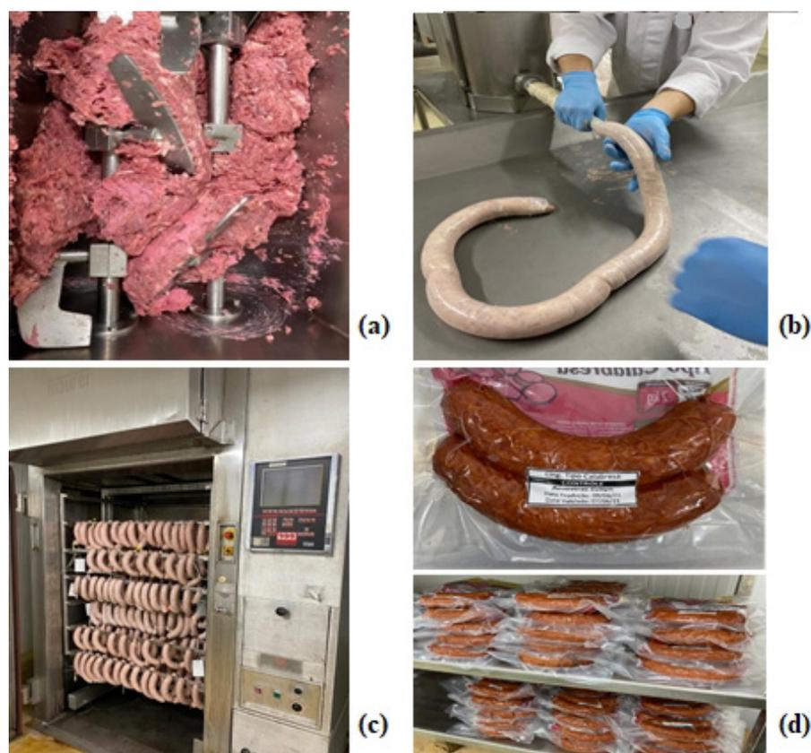
**Figure 1.** Illustration of industrial processes of mixing (a), stuffing (b), cooking (c), and packaging (d) of Calabrese-type sausages.
