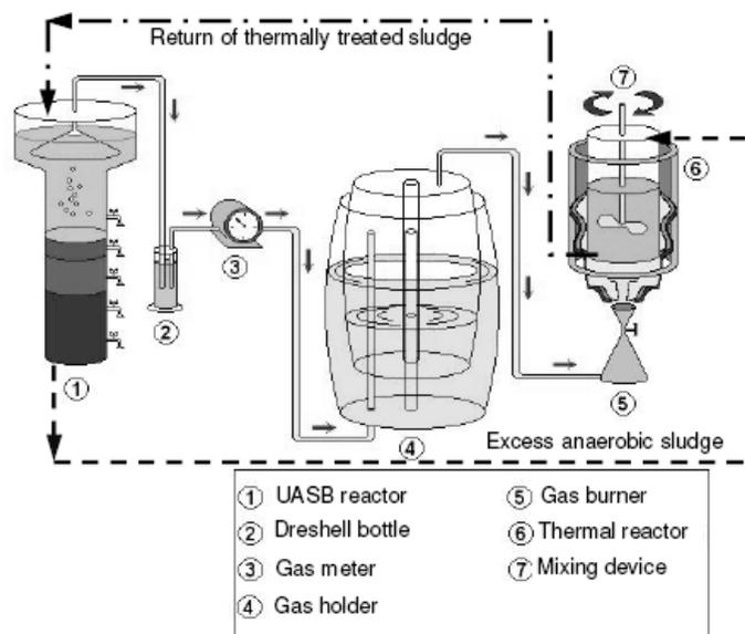
**Figure 1:** Set up of the experimental apparatus
