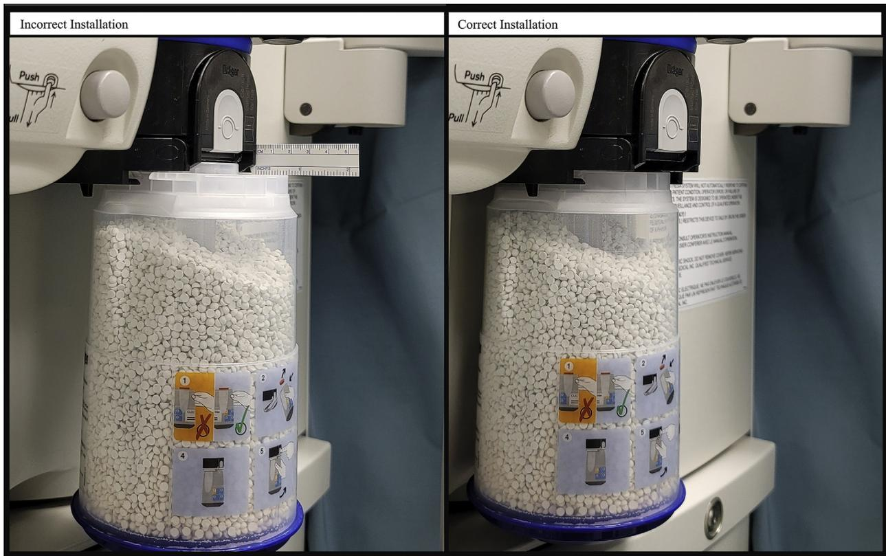
**Figure 1** Installation of the carbon dioxide absorbent canister.
