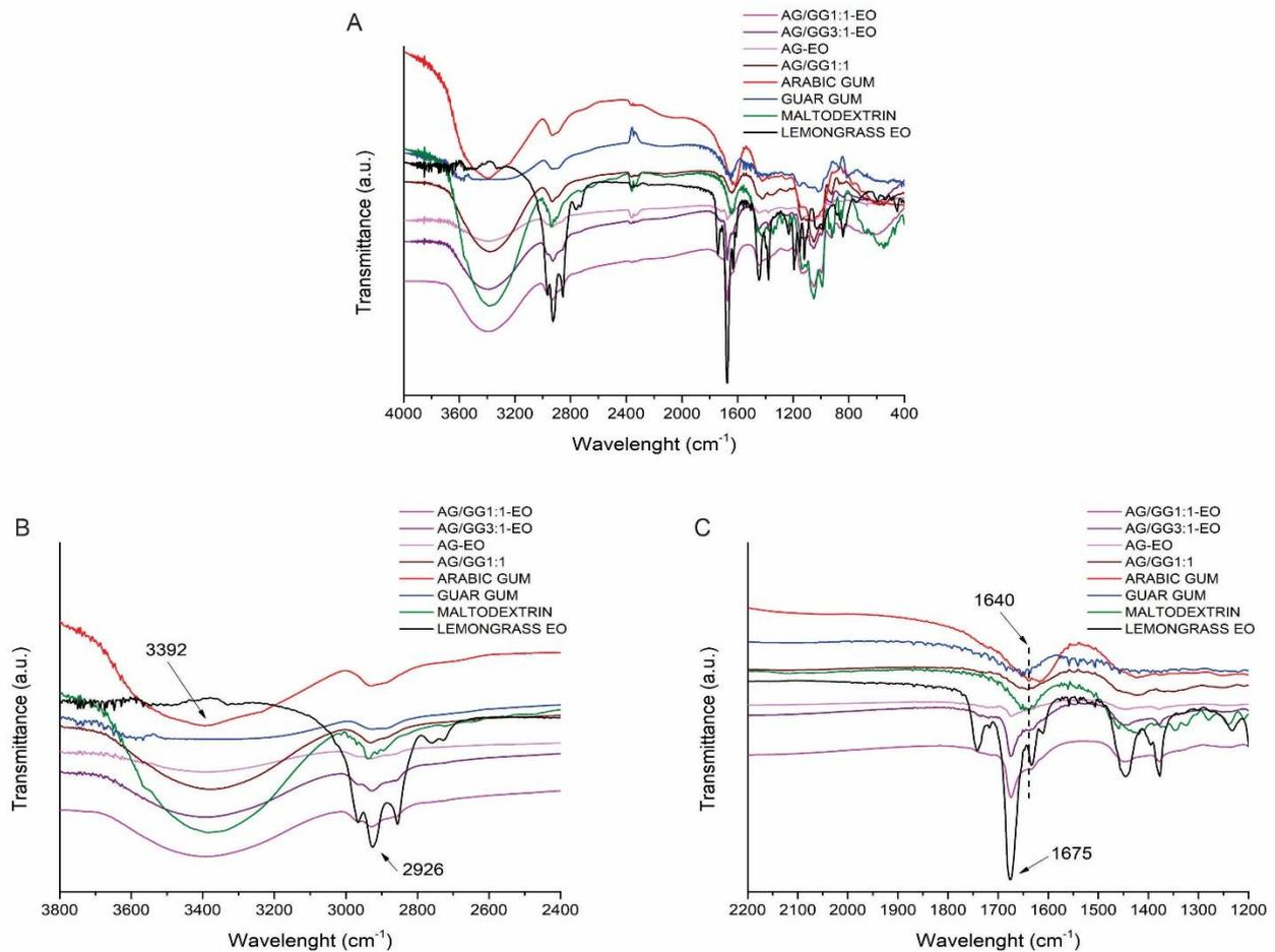
**Figure 3.** FTIR spectra of lemongrass essential oil, encapsulating agents, and microparticles. (A) over the range 4000-400  $\text{cm}^{-1}$ , (B) over the range 3800-2400  $\text{cm}^{-1}$ , and (C) over the range 2200-1200  $\text{cm}^{-1}$ .
