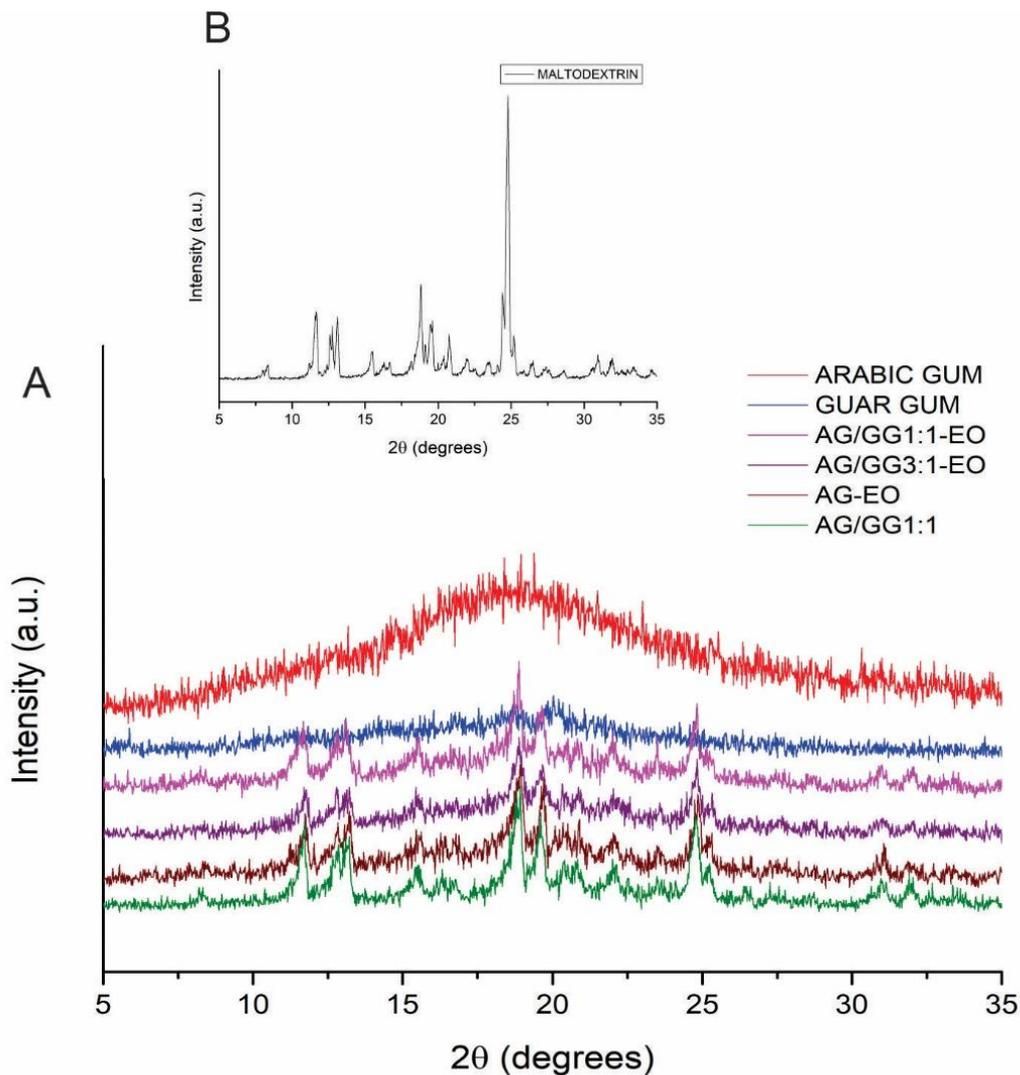
**Figure 4.** XRD diffractogram of (A) microparticles and encapsulating agents; (B) maltodextrin.
