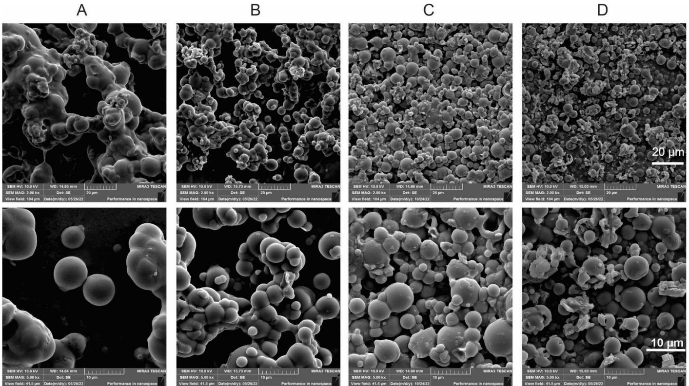
**Figure 2.** FEG-SEM micrographs of microparticles. (A) AG/GG1:1-EO, (B) AG/GG3:1-EO, (C) AG-EO, (D) AG/GG1:1 (control). First line: 20 µm; 2,000 x; second line: 10 µm; 5,000 x.
