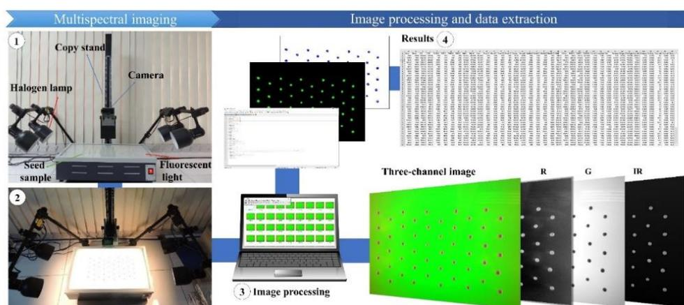
**Figure 1.** System for multispectral image acquisition and image processing. Overview of the equipment for image acquisition (1); sample of seeds placed on the system (2); image segmentation and processing using ImageJ<sup>®</sup> software (3); and table of results following the analysis (4).
