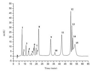
**Figure 1.** Chromatogram of the phenolic acid standard solution with spectrophotometric detection at 280 nm. Identified peaks: 1 = Gallic acid; 2 = gallocatechin; 3 = 3,4 dihydroxy phenolic 4 = catechin; 5 = chlorogenic acid; 6 = epigallocatechin; 7 = vanillic acid; 8 = syringic acid; 9 = P-coumaric acid; 10 = ferulic acid; 11 = M-coumaric acid; 12 = O-coumaric acid; 13 = Resveratrol; 14 = ellagic acid and 15 = Salicylic acid.
