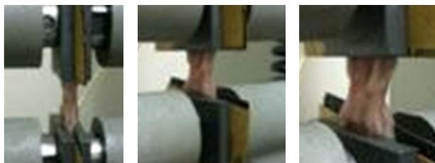
**Figure 2** - Tissues were placed in the jaws of the device with the incision line in the middle and the tension force was applied at a speed of 10 mm/min until the tissues were broken. The tensile strength was obtained by using the Instron Series IX Automated Material Testing System Version 5.33 device.
