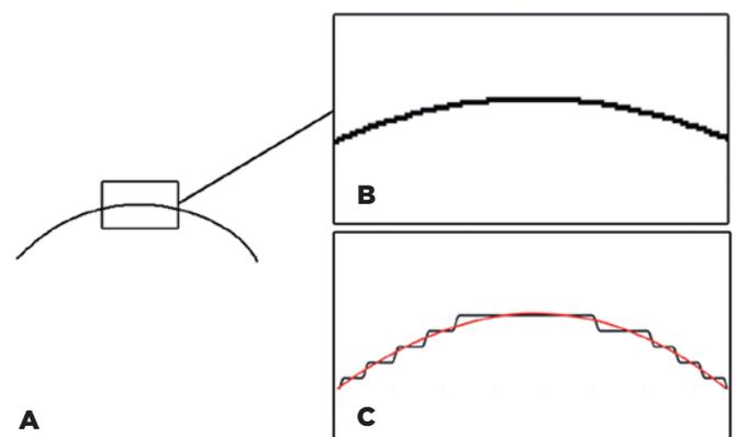
**Figure 2.** A) Black line after binarization of the yellow Bézier line. B) Upper, small irregularities due to pixel dimension. C) Effect of smoothing the curve using a Savitzky-Golay filter.
