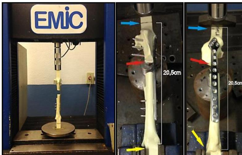
Figure 2. Mechanical configuration used for compression (A) and three-point craniocaudal (B) and mediolateral bending testing (C) of constructs. Yellow arrow: distal block secured in a vice; red arrow: support on the lateral surface of the specimen 45 mm from the tibial plateau; blue arrow: location where the testing machine applied force.
